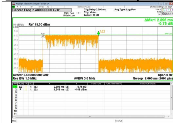
Pulse Width 8DPSK_3-DH5
