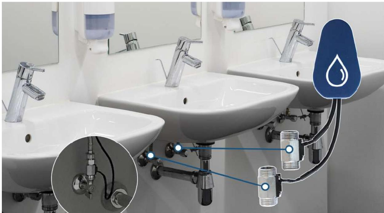
Then, on the **asset configuration page**, you can specify which sensor is measuring which water stream.
