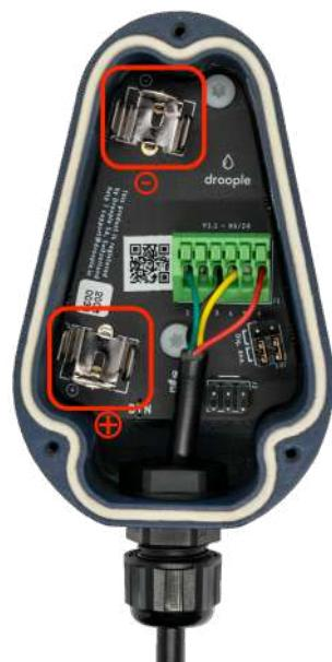
3. Place the battery inside the connectors and make sure that the indicated polarities match the ones from the battery.
