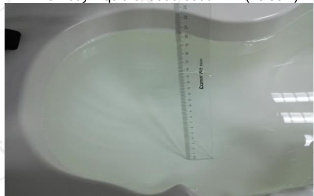
The Head Liquid of 5000-6000MHz (15.8cm)
