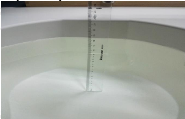
The Body Liquid of 2450MHz (15.3cm)
