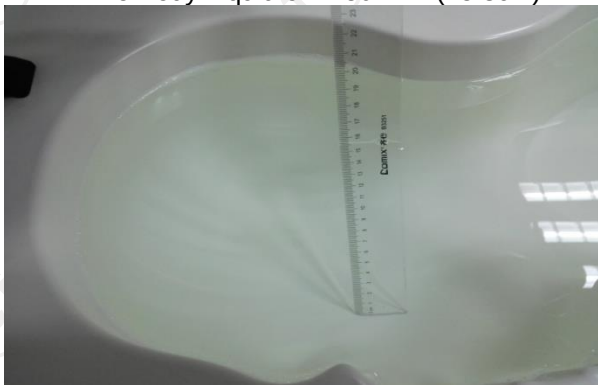
The Head Liquid of 2450MHz (15.6cm)
