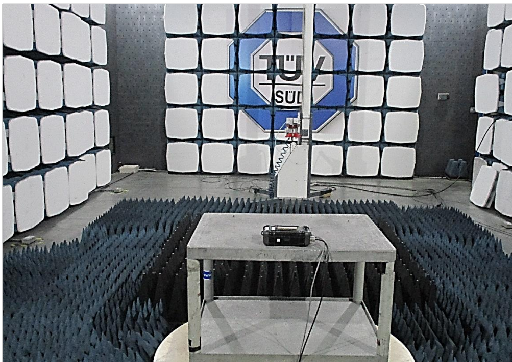
Figure 23 - Test Setup - 1 GHz to 12.5 GHz - X Orientation
