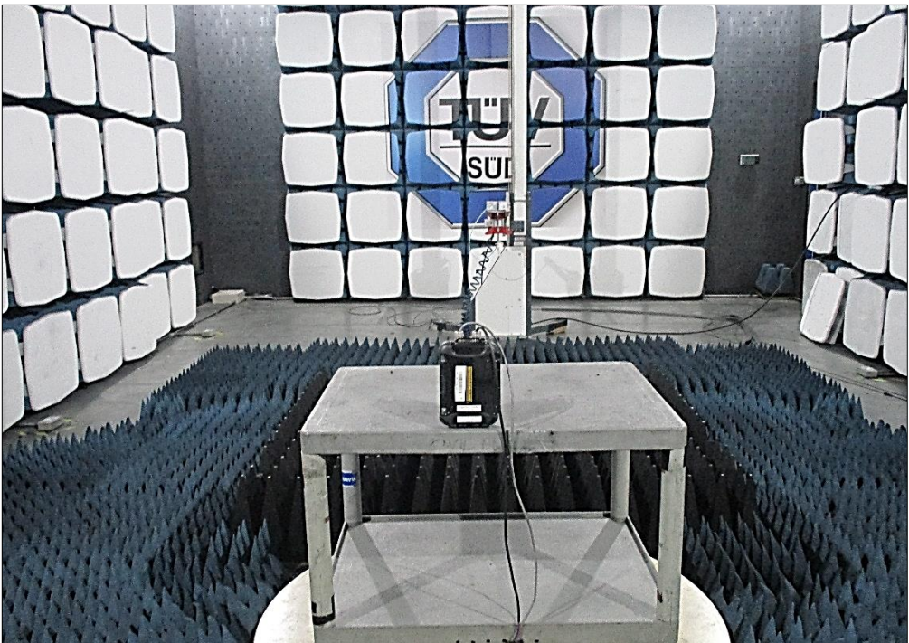
Figure 27 - Test Setup - 1 GHz to 12.5 GHz - Z Orientation
