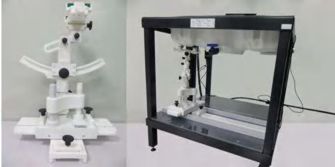
Device holder supplied by SATIMO
