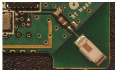
Then the wire antenna is installed on to the DWE-DML1 module as shown below.
