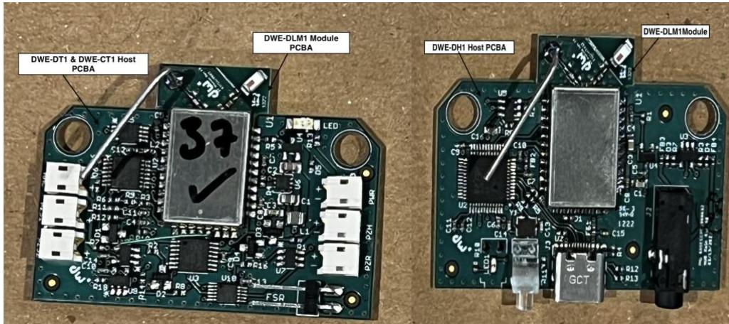
The module/host PCBAs are now ready to install into their respective host mechanics to complete final host assembly.
