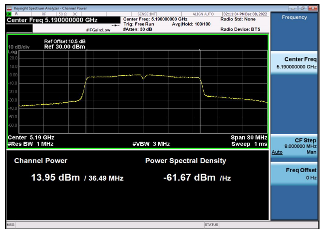
U-NII-1 Output Power-802.11a(20MHz) ,5180MHz,Ant1
