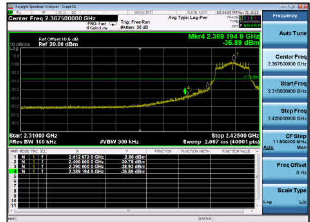
,Plot 2,Band Edge-802.11g,2462MHz ,Ant0
