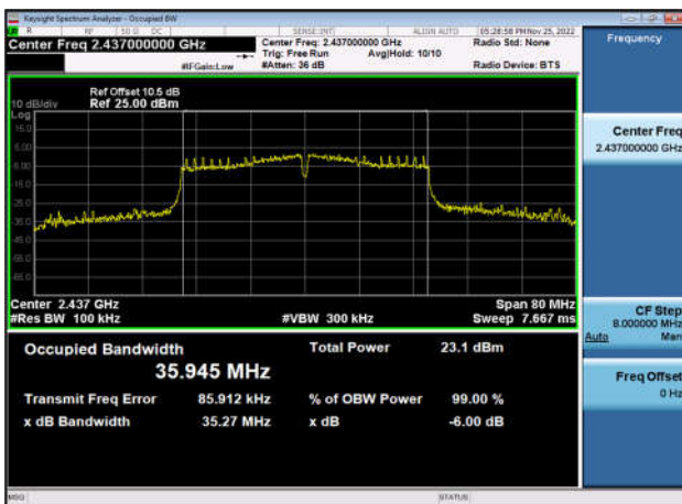
6dB Bandwidth-802.11n(HT40),2437MHz ,Ant0
