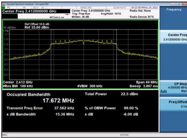
6dB Bandwidth-802.11n(HT20),2462MHz ,Ant0
