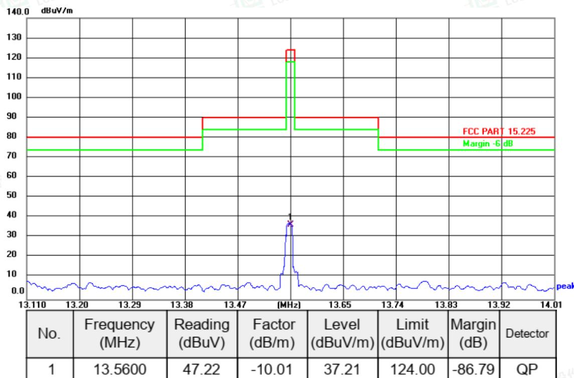
\*Note: Factor= Antenna Factor + Cable Loss
