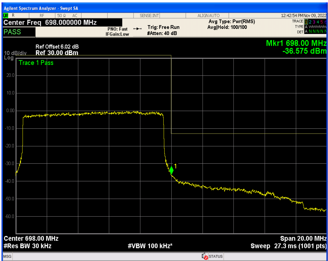
Band71 QAM16 BW=10MHz Channel=133422 RB Size=1 Position=#0
