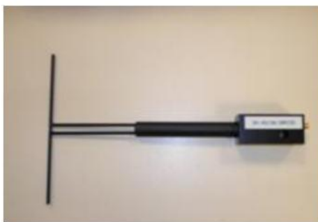
Figure 1 – Satimo COMOSAR Validation Dipole
