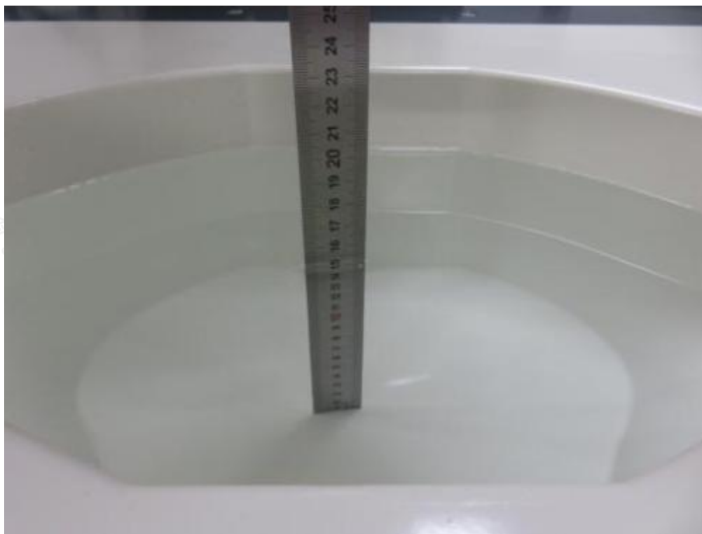
Photograph of the depth in the Head Phantom (2450MHz, 15.1cm depth)
