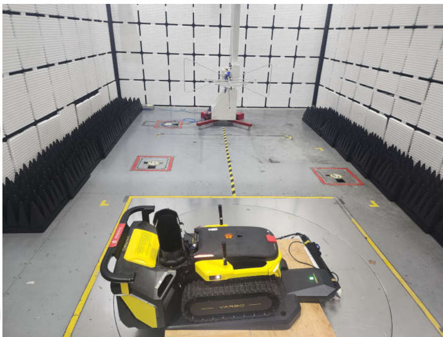
Radiated Emissions Test Setup (30MHz-1GHz)
