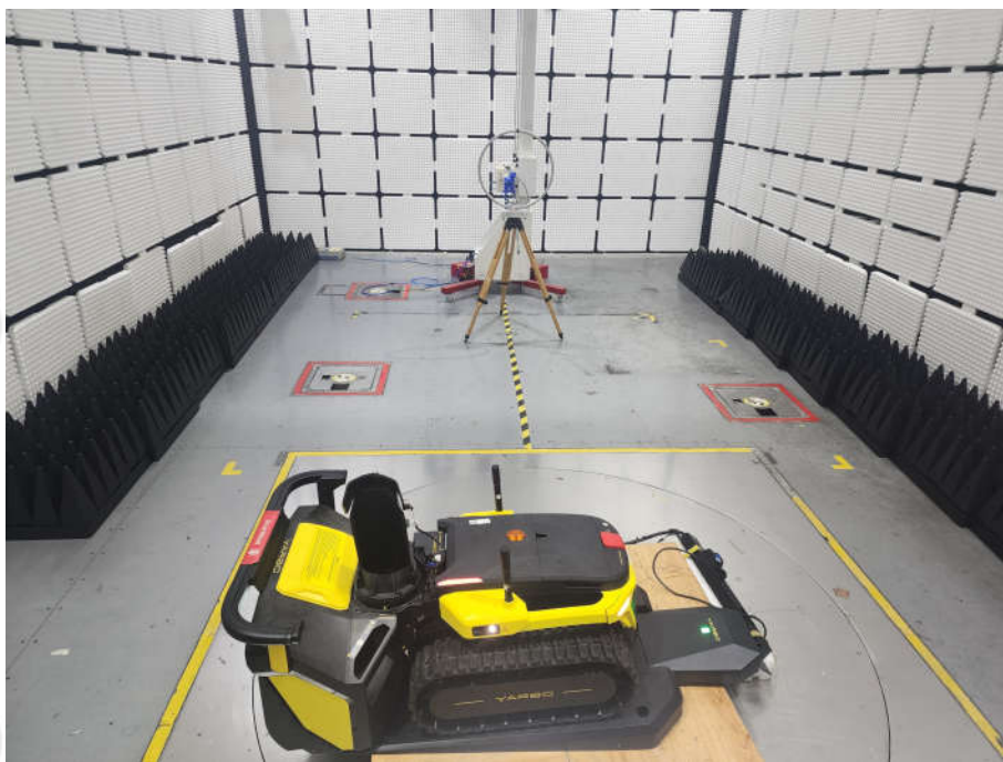
Radiated Emissions Test Setup (9kHz-30MHz)
