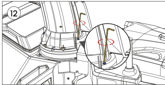
**Tighten** the 2 bolts on the edge first with Allen Key #2
