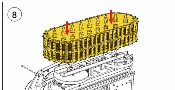
Locate the Snow Track provided in the package and install the Snow Track. Please ensure the track direction is correct as shown in the picture.
