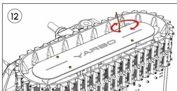
Place back the Side Panel and screw the four bolts to tighten the panel using Allen Key#2.
