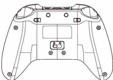
Make sure that the slide switch is slid to the left side.
