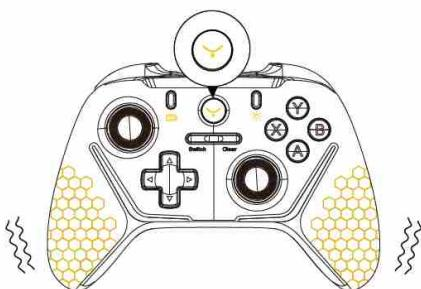
Press and hold the Yarbo Logo Button for approximately 5 seconds to turn on the physical controller and initiate the pairing mode.
