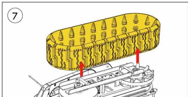
Tap both ends of the track and carefully detach the track from the Yarbo Core. If it is still too hard to detach the track, please repeat step 4 and step 5.
