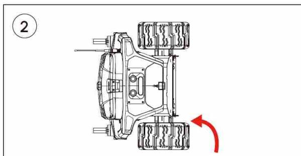
Rotate the Yarbo Core to a vertical position on its side.
