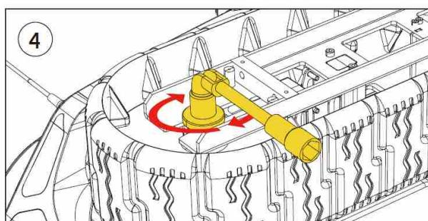
Locate L-Shaped Socket Wrench for Track provide in the package and use this tool to loosen the bolt shown in the picture.
