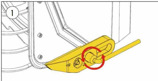
Locate Socket #2, which is provided in the package, and find the location for the skid shoes.
