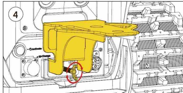
Locate the tow hitch bolt provided in the package and tighten the tow hitch by screwing the bolt. Ensure that the bolt is securely fastened to prevent any loosening while towing.
