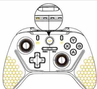
Observe the LED light on the top of Yarbo Controller. If the left yellow light is on steadily, it indicates that connected with the phone.
