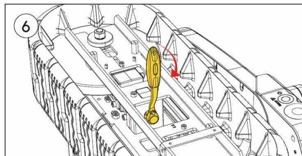
Locate the Track Wrench in the package and loosen the bolt shown in the picture.
