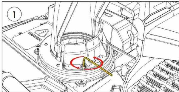
**Unscrew** and Remove the two Snow Plume Diverter connection bolts using Allen Key #2.
