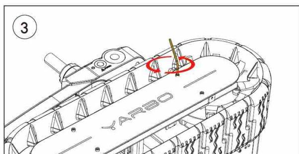
Remove the Side Panel by unscrewing the four bolts shown in the picture using Allen Key#2.
