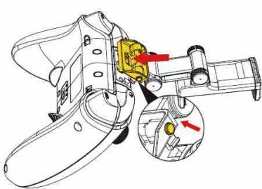
Locate the shafts and holes and press the buttons on both sides of the Holder, and then press the middle part as shown in the picture.
