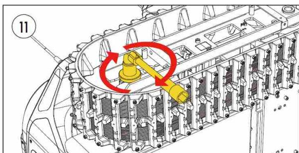
Locate L-Shaped Socket Wrench for Track and use the tool to tighten the track.
