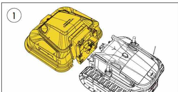
Please remove the module in the front for better adjusting the track.
