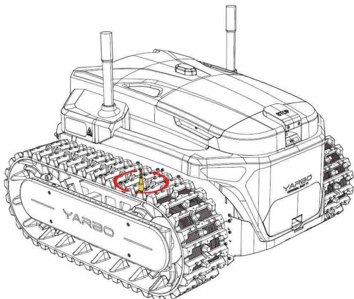
**Loosen** all the anti-slip studs on the track with Socket #1 or any electronic tools(not provided).
