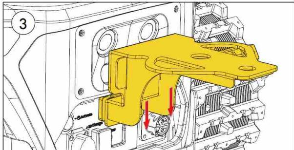
Slide the tow hitch down to the bottom of the mount.
