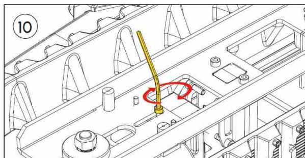
Tighten the bolt using Allen Key#4
