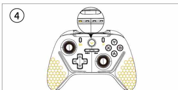
Observe the LED light on the top of Yarbo Controller. If the yellow light is on steadily, it indicates that the physical controller has been successfully connected.
