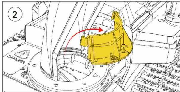
**Remove** the Snow Plume Diverter.
