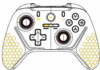
To gain the authority of physical controller, hold the Switch button for 2-3s to gain the authority. Once Yarbo gains authority, you can control the yarbo now.
