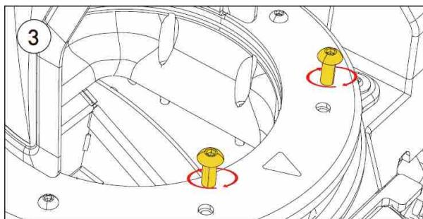
Tighten the two Snow Plume Diverter connection bolts just removed.
