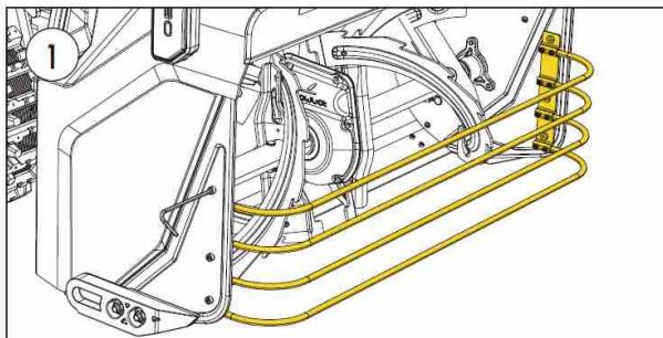
**Unscrew** the bolts in both sides of the protection fence using Allen Key #2 provided in the package.
