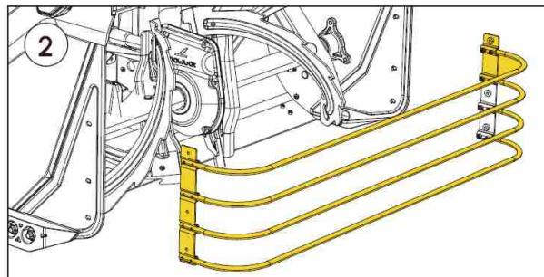
**Remove** the protection fence and safely preserve the bolts and fence.
