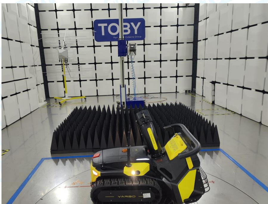
Photo of Setup for Radiated Emission (Above 1 GHz)
