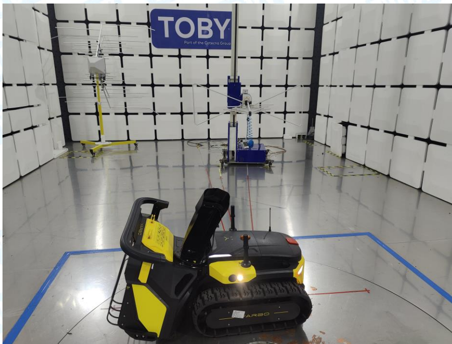
Photo of Setup for Radiated Emission (Above 1 GHz)
