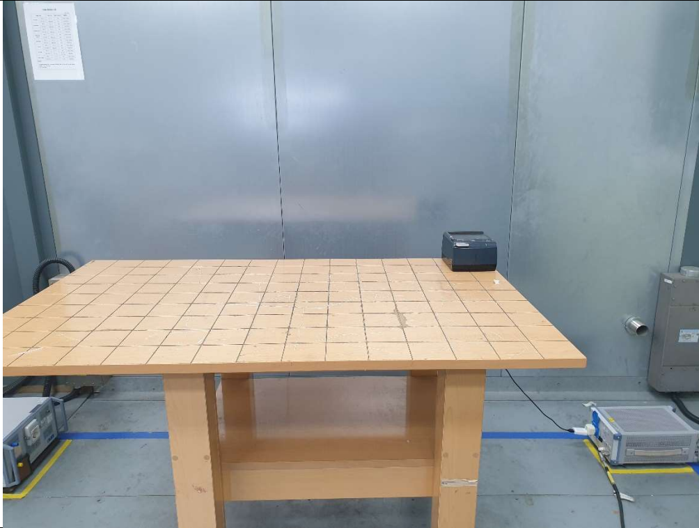
AC power line conducted emissions_Rear
