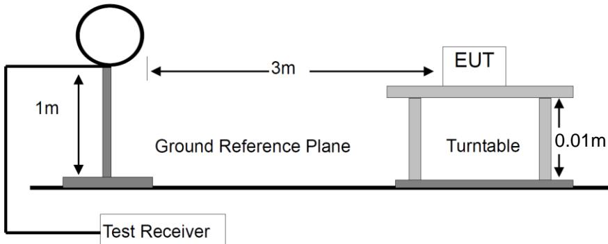
For Radiated Emission 30-1000MHz
