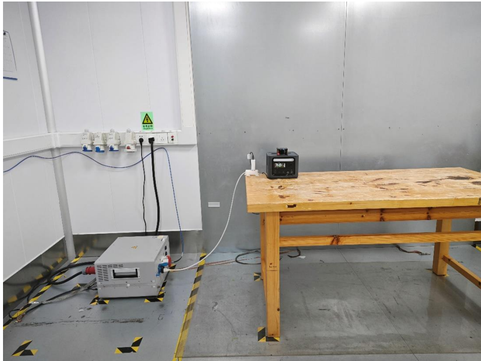
Photograph 3: Set-up photo for Conducted Emission
