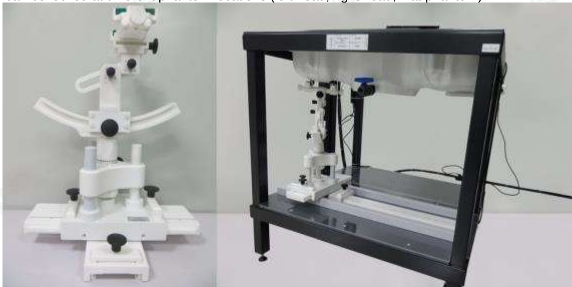
Device holder supplied by SATIMO
