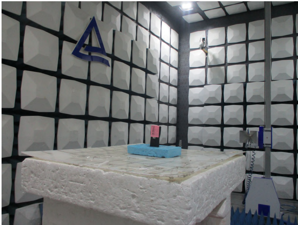
Photograph 2: Set-up for Radiated Spurious Emission, 1GHz - 18GHz
