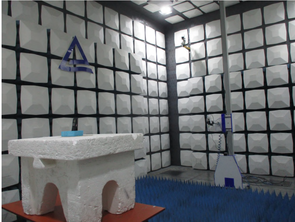
Photograph 3: Set-up for Radiated Spurious Emission, 18GHz - 26.5GHz
