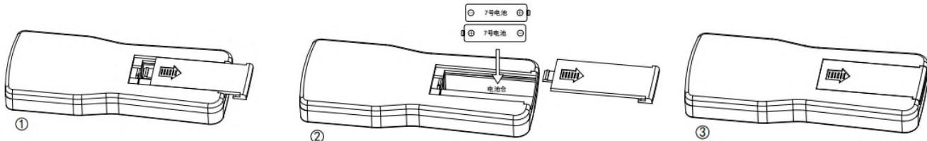
Step 1: Slide off the battery cover via the arrow direction
