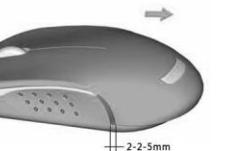
C, Once the upper cover is removed, Install the battery inside. The receiver can be placed on the middle shell.
