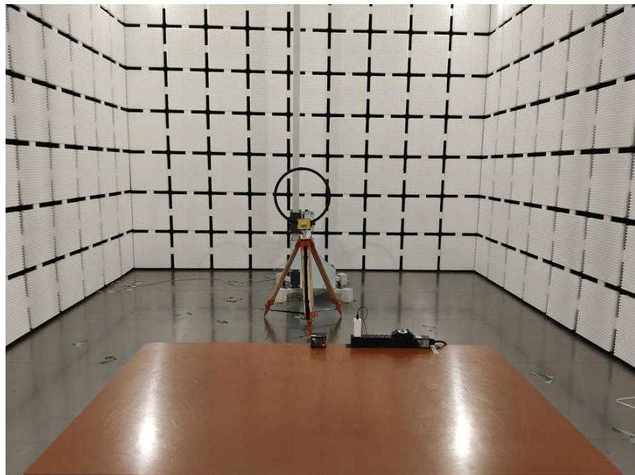
**Radiated Emission Test View 30MHz-1GHz**
