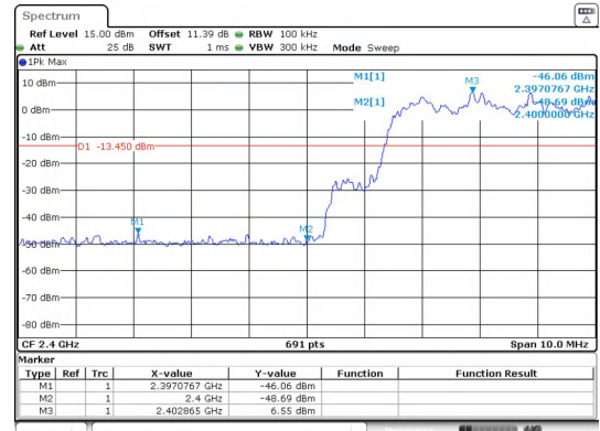
Out Of Band Emission(Left) \pi/4 DQPSK_2-DH5_Channel Hopping
