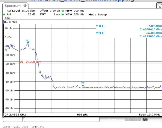
Out Of Band Emission(Right) \pi/4 DQPSK_2-DH5_Channel Hopping
