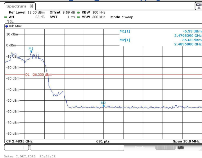
Out Of Band Emission(Right) 8DPSK_3-DH5_Channel Hopping
