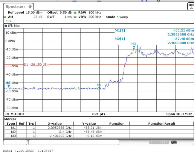
Out Of Band Emission(Left) \pi/4 DQPSK_2-DH5_Channel Hopping
