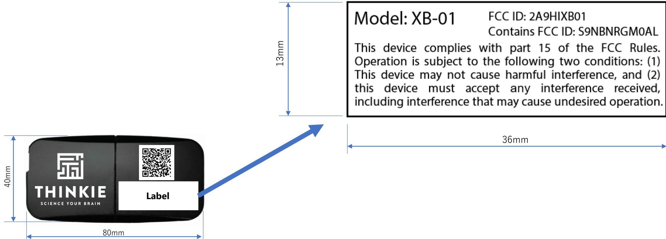
The FCC ID label is permanently affixed on the device with an adhesive.
