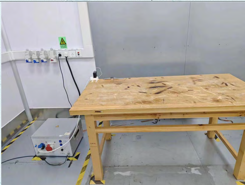
Conducted Emission at AC power line
