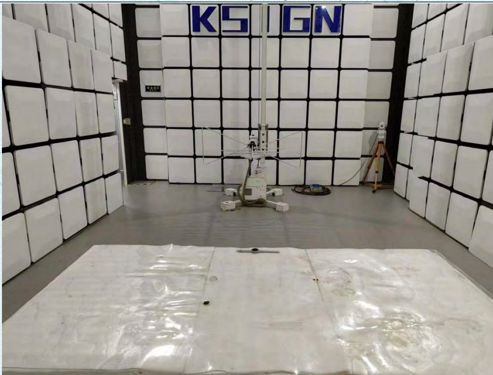
Emissions in restricted frequency bands (below 1GHz)
