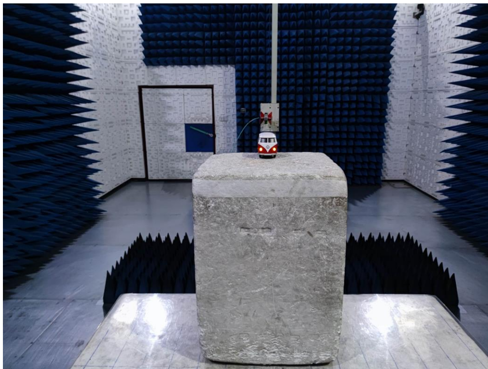
RADIATED EMISSION TEST SETUP ABOVE 1GHz
