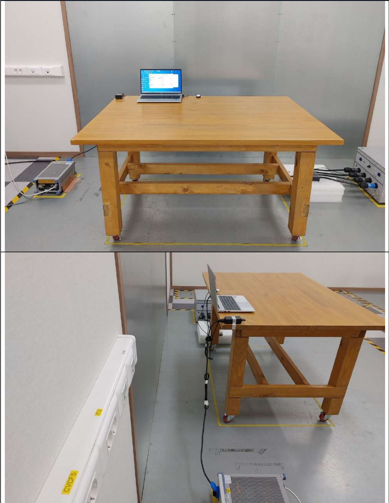
Photo of test set up for conducted voltage emissions Test configuration: Configuration #2 (Data transmitting_1 Port)
