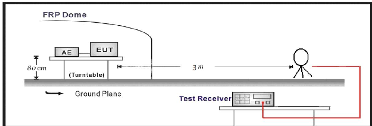
Below 1GHz Test Setup:
