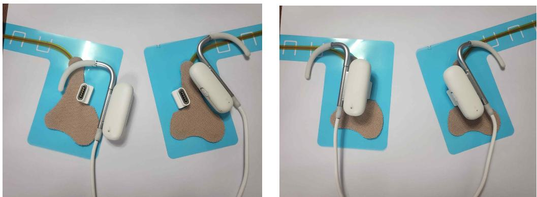
2. Turn on the switch on the right side device. If device turn on, the Blue LED blink.
