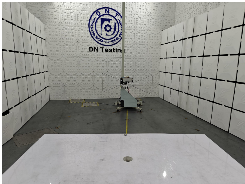
Radiated Emission Test View (Below 1G)
