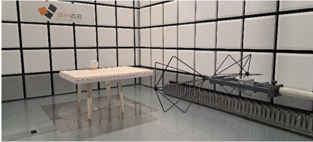
Measurement < 1GHz, in semi anechoic room
