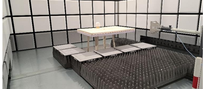
Measurement > 1GHz, in full anechoic room (semi anechoic room with RF absorbers on the floor)
