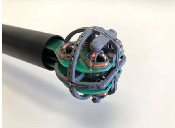
Test probe, without the casing
