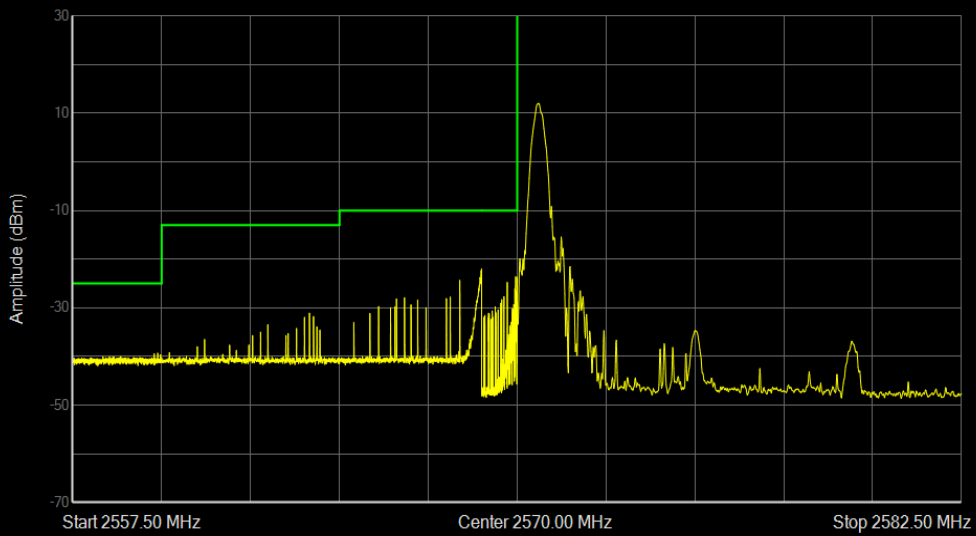
Band38 QAM16 BW=10MHz Channel=37800 RB Size=1 Position=#0
