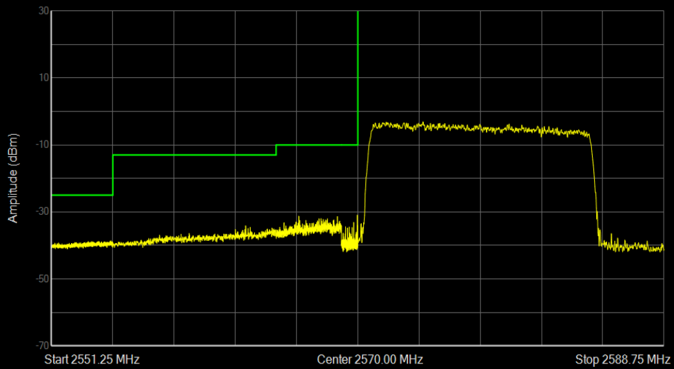
Band38 QAM16 BW=15MHz Channel=37825 RB Size=75 Position=#0
