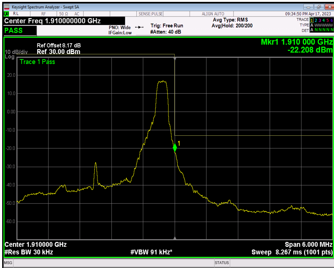
Band2 QPSK BW=3MHz Channel=19185 RB Size=15 Position=#0
