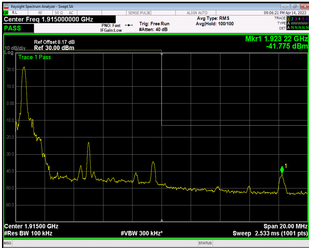
Band25 QPSK BW=10MHz Channel=26640 RB Size=1 Position=#Max
