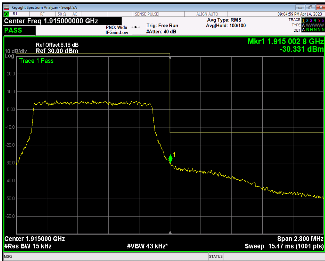
Band25 QPSK BW=3MHz Channel=26055 RB Size=1 Position=#0
