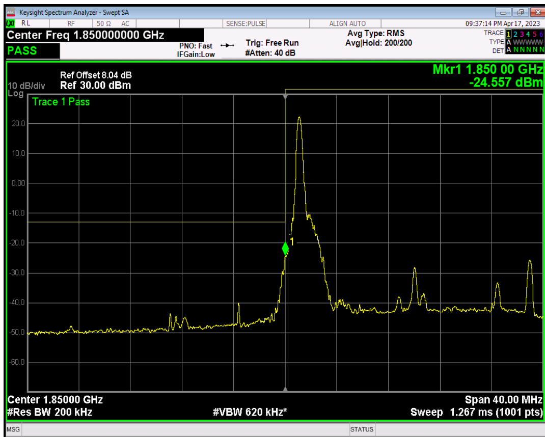
Band2 QAM16 BW=20MHz Channel=18700 RB Size=1 Position=#Max
