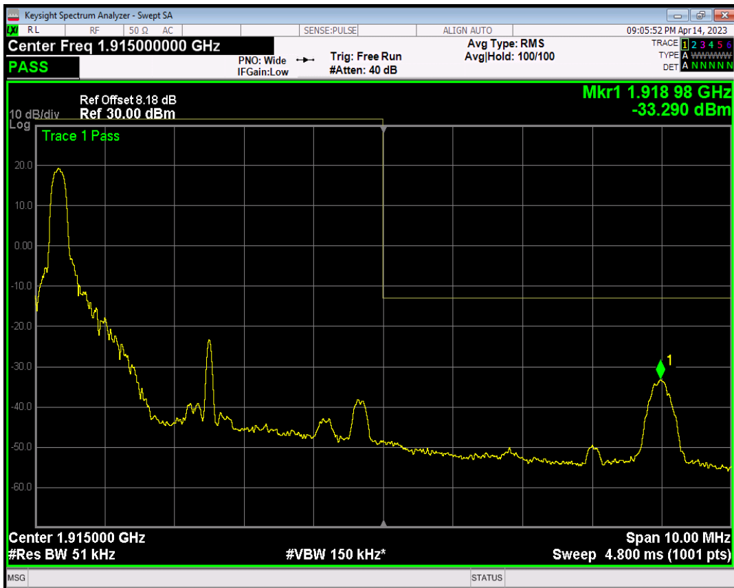
Band25 QPSK BW=5MHz Channel=26665 RB Size=1 Position=#Max
