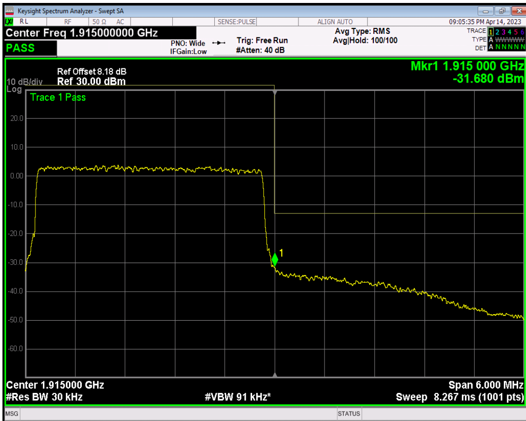
Band25 QPSK BW=5MHz Channel=26065 RB Size=1 Position=#0
