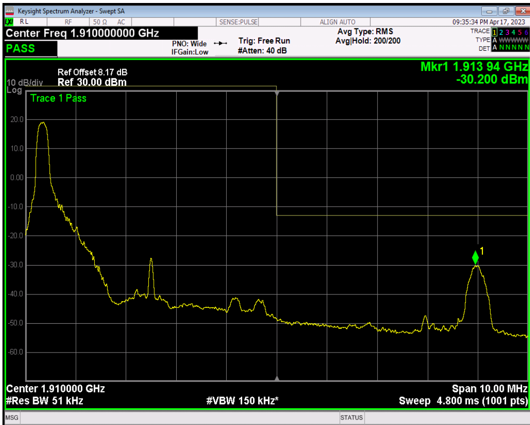
Band2 QPSK BW=5MHz Channel=19175 RB Size=25 Position=#0
