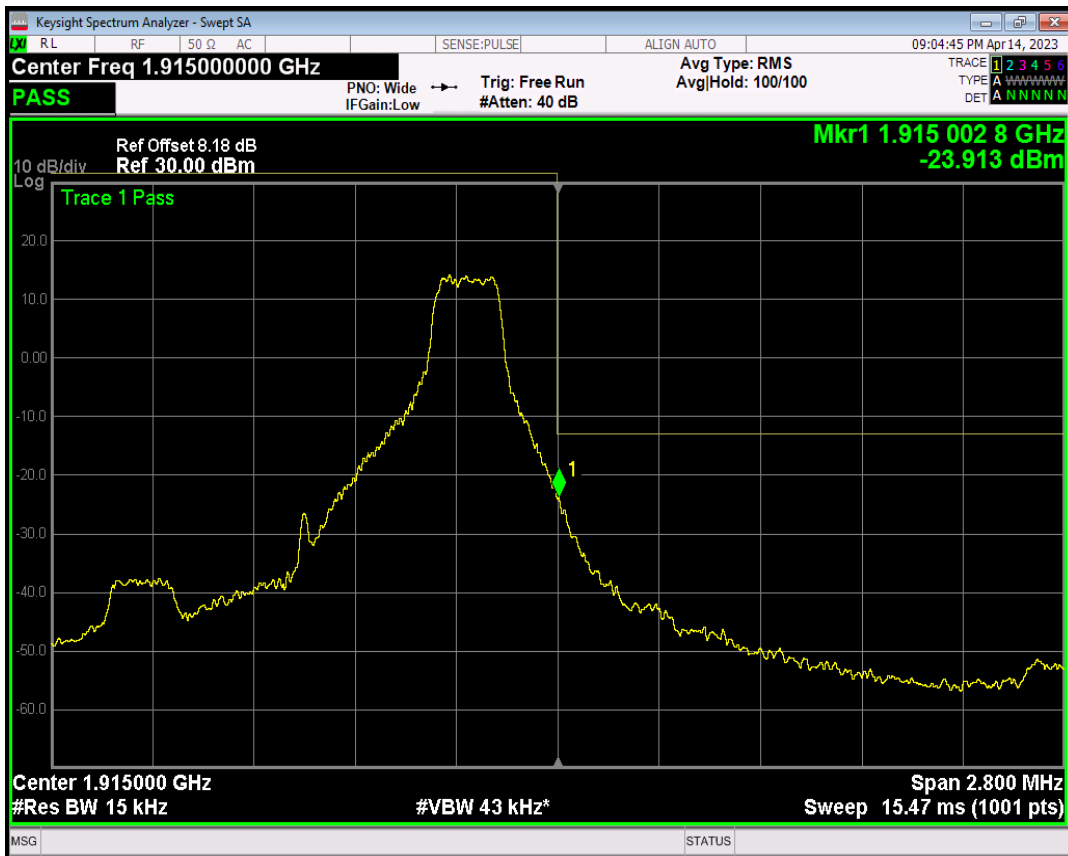
Band25 QPSK BW=1.4MHz Channel=26683 RB Size=6 Position=#0
