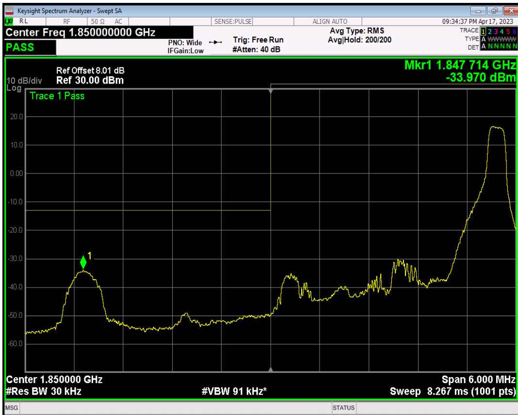
Band2 QAM16 BW=3MHz Channel=18615 RB Size=15 Position=#0
