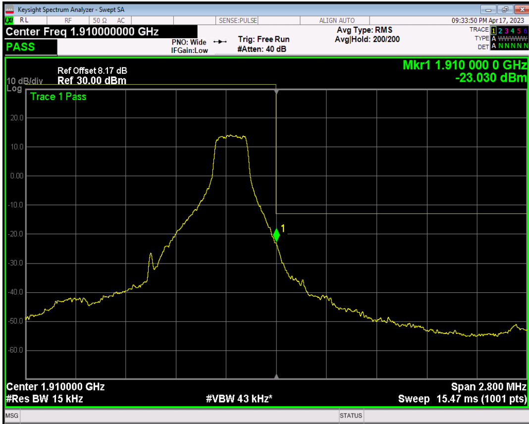
Band2 QPSK BW=1.4MHz Channel=19193 RB Size=6 Position=#0
