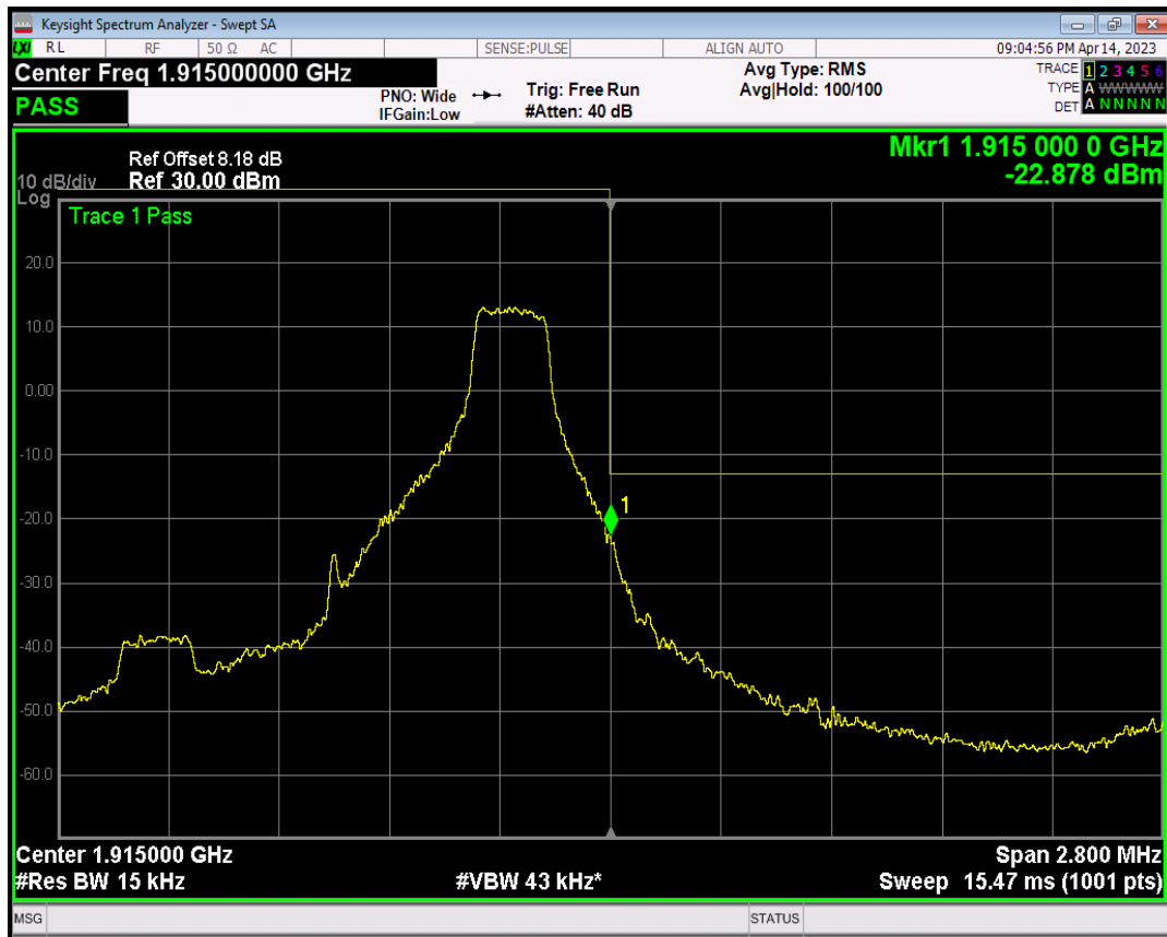
Band25 QAM16 BW=1.4MHz Channel=26683 RB Size=6 Position=#0
