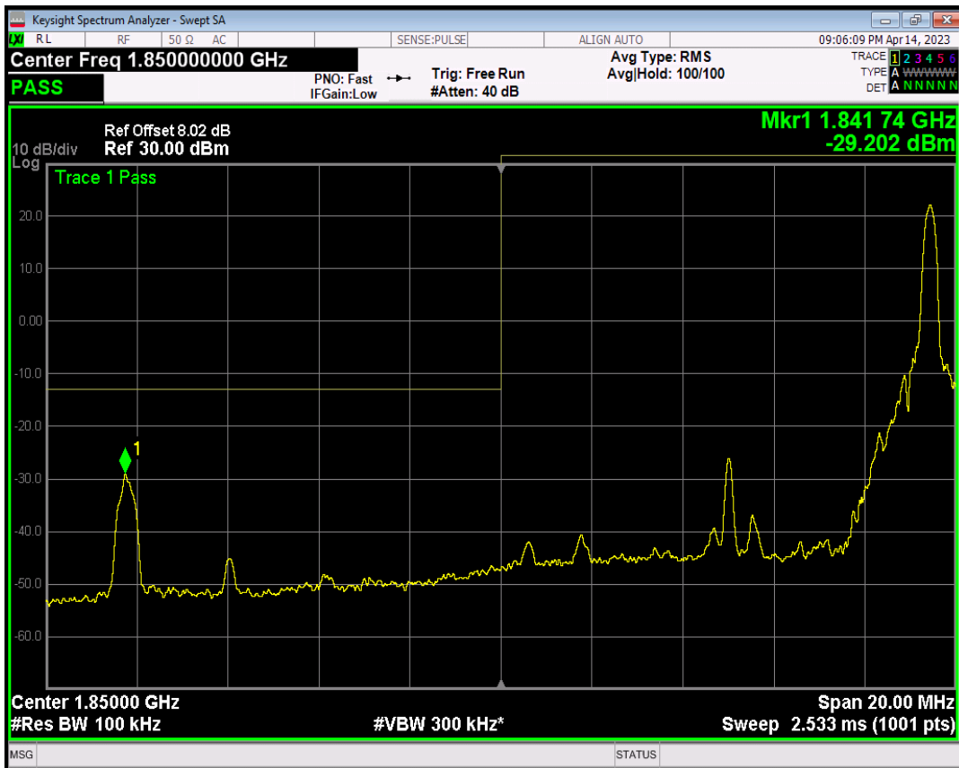
Band25 QPSK BW=10MHz Channel=26090 RB Size=50 Position=#0
