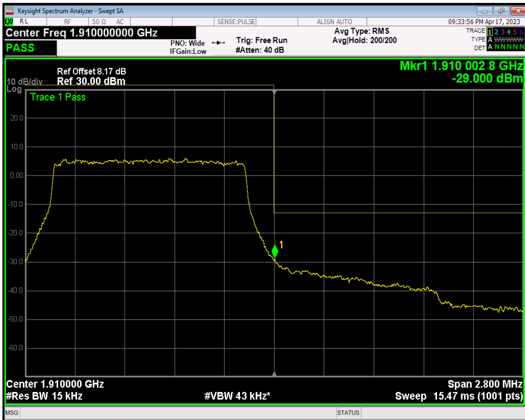
Band2 QAM16 BW=1.4MHz Channel=19193 RB Size=1 Position=#0
