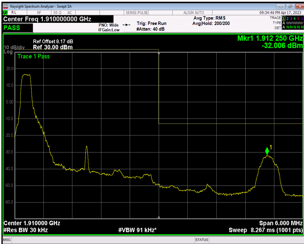
Band2 QPSK BW=3MHz Channel=19185 RB Size=1 Position=#Max
