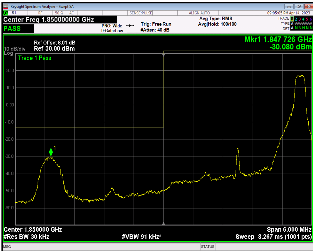
Band25 QPSK BW=3MHz Channel=26055 RB Size=15 Position=#0
