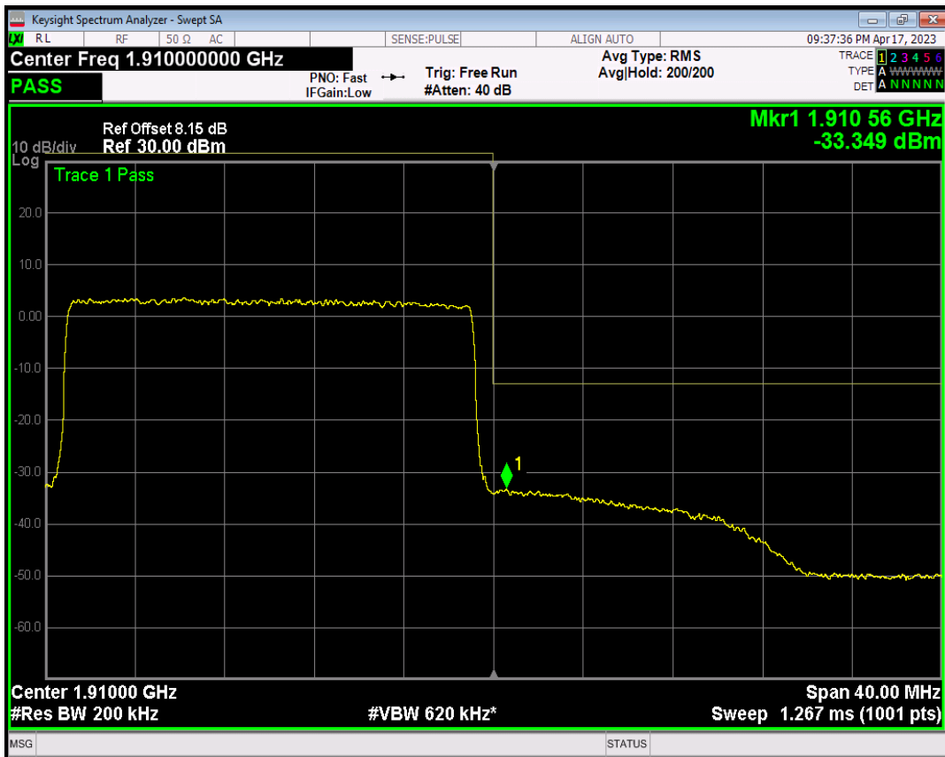
Band25 QPSK BW=1.4MHz Channel=26047 RB Size=1 Position=#0
