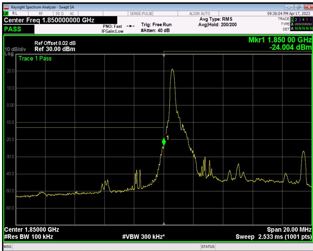
Band2 QAM16 BW=10MHz Channel=18650 RB Size=1 Position=#Max
