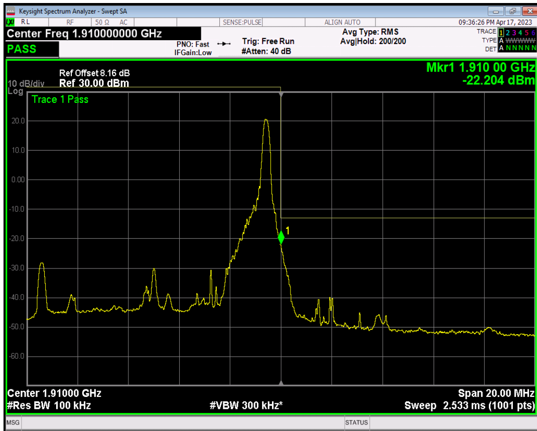
Band2 QAM16 BW=10MHz Channel=19150 RB Size=50 Position=#0
