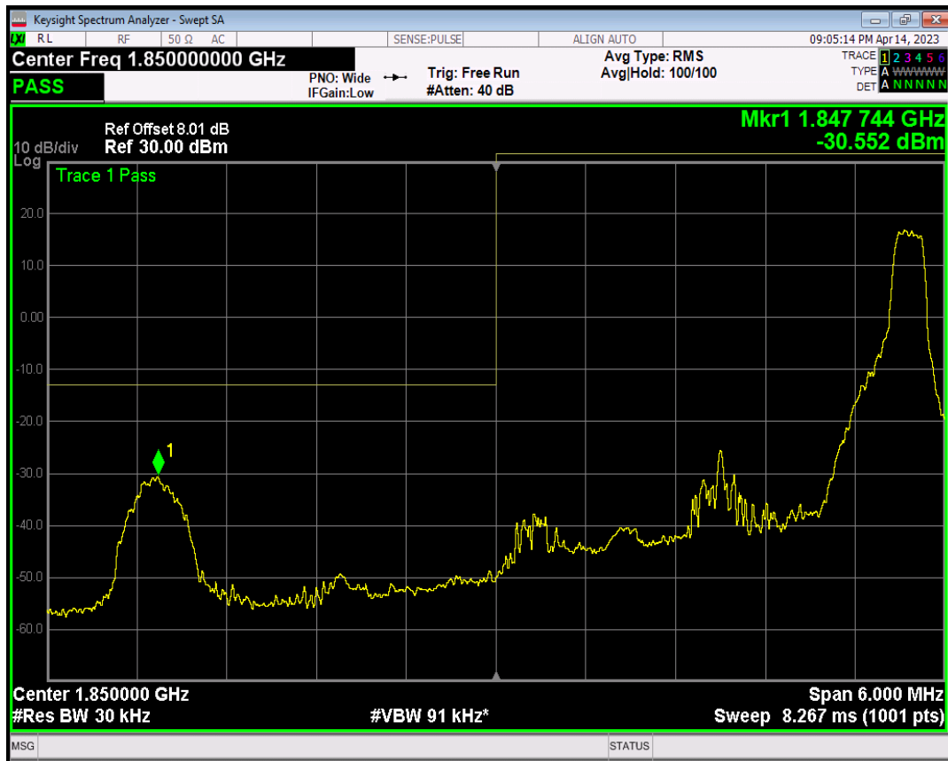
Band25 QAM16 BW=3MHz Channel=26055 RB Size=15 Position=#0
