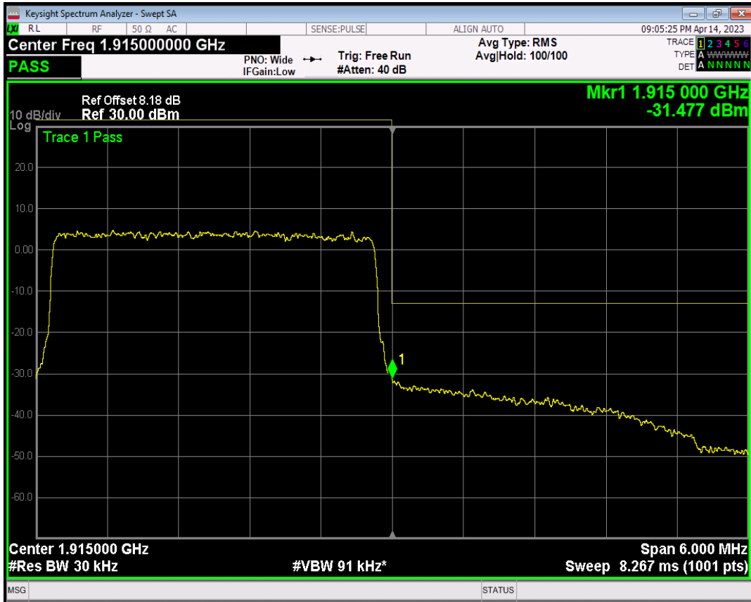
Band25 QAM16 BW=3MHz Channel=26675 RB Size=1 Position=#0
