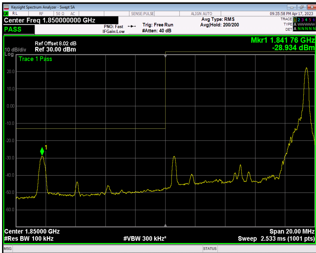
Band2 QPSK BW=10MHz Channel=18650 RB Size=50 Position=#0
