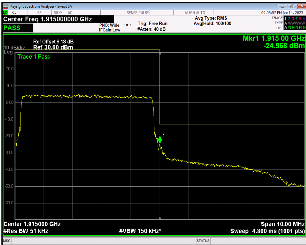
Band25 QAM16 BW=5MHz Channel=26665 RB Size=1 Position=#0
