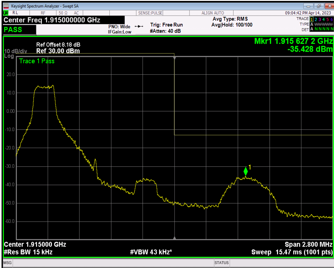
Band25 QPSK BW=1.4MHz Channel=26683 RB Size=1 Position=#Max
