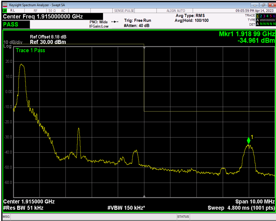
Band25 QAM16 BW=5MHz Channel=26665 RB Size=25 Position=#0
