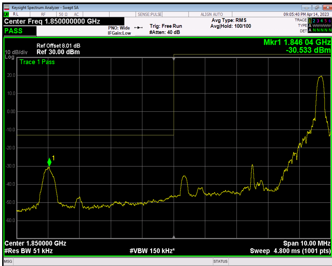
Band25 QPSK BW=5MHz Channel=26065 RB Size=25 Position=#0
