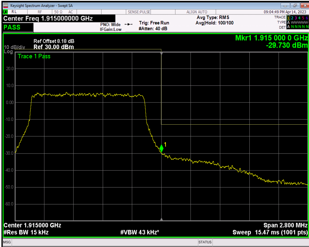
Band25 QAM16 BW=1.4MHz Channel=26683 RB Size=1 Position=#0
