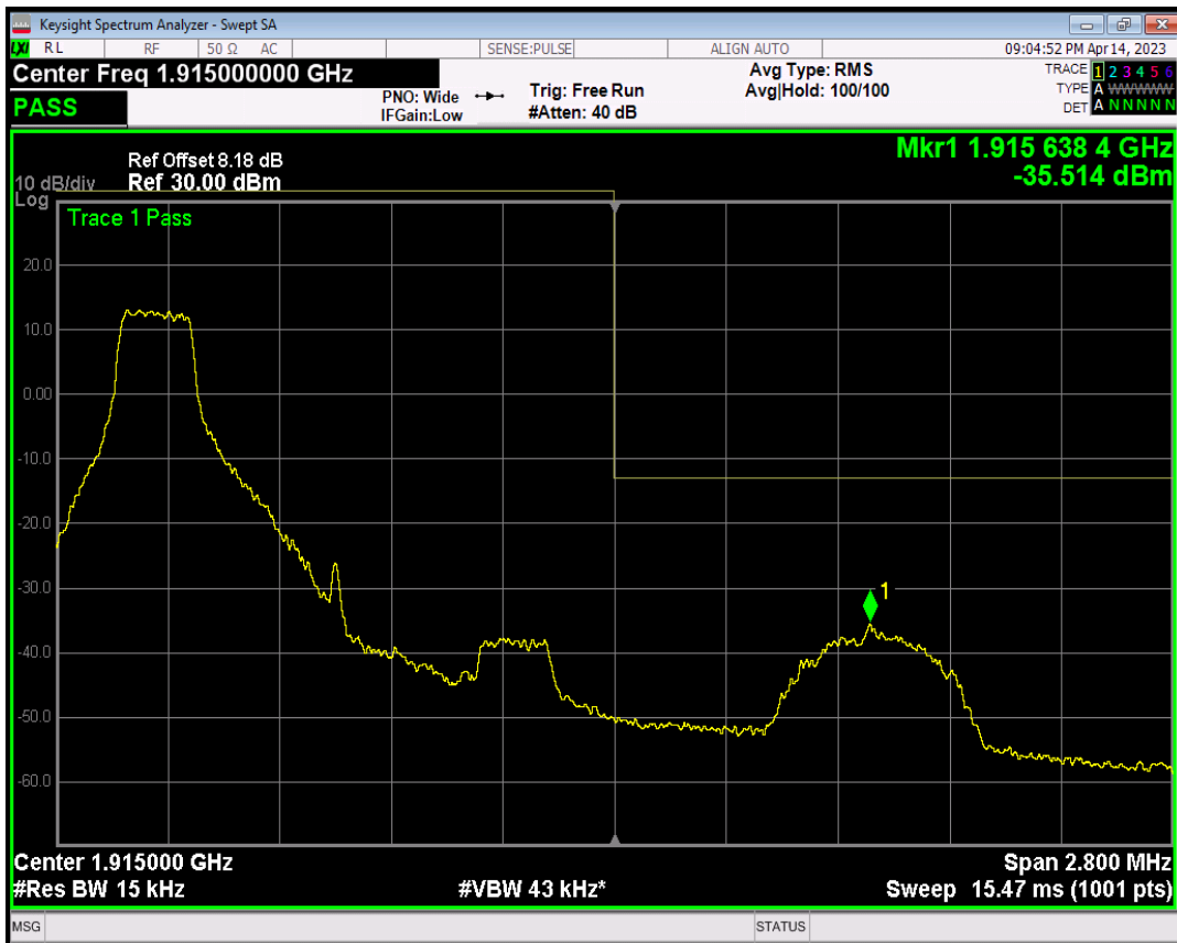
Band25 QAM16 BW=1.4MHz Channel=26683 RB Size=1 Position=#Max
