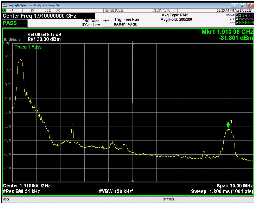
Band2 QAM16 BW=5MHz Channel=19175 RB Size=1 Position=#Max
