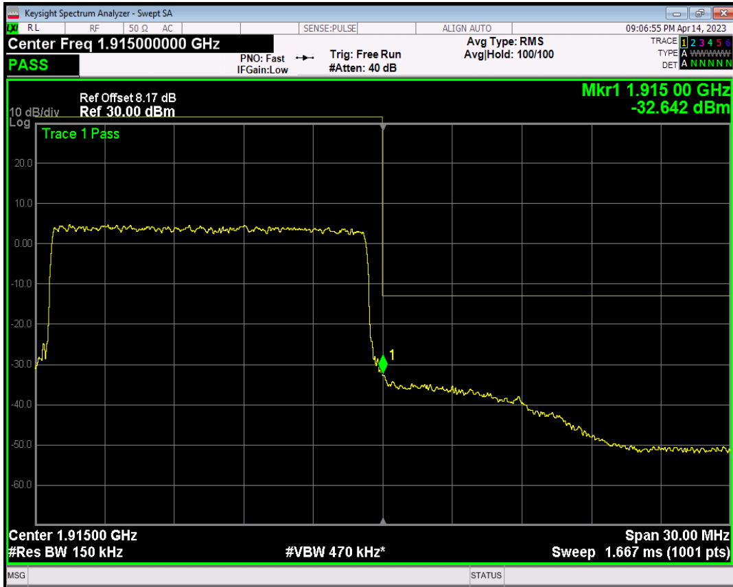
Band25 QAM16 BW=15MHz Channel=26615 RB Size=1 Position=#0
