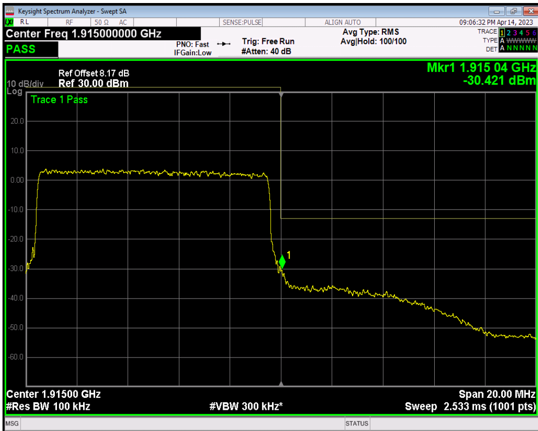
Band25 QPSK BW=15MHz Channel=26115 RB Size=1 Position=#0
