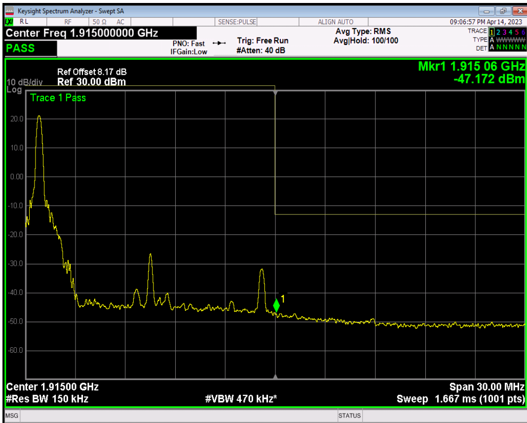
Band25 QAM16 BW=15MHz Channel=26615 RB Size=1 Position=#Max
