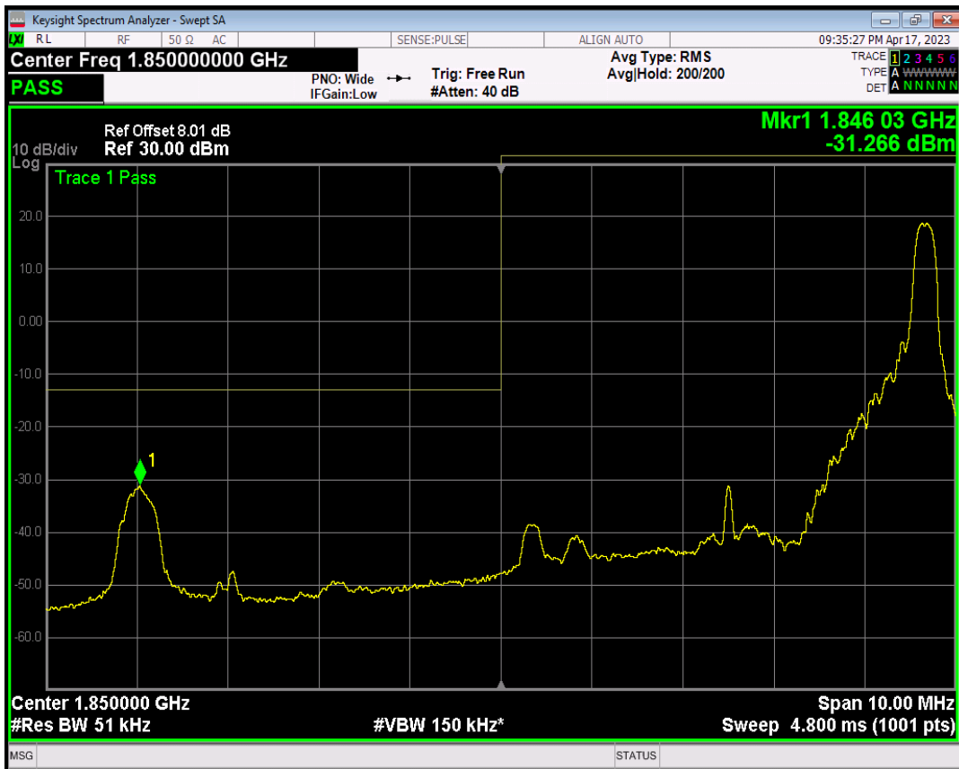
Band2 QAM16 BW=5MHz Channel=18625 RB Size=25 Position=#0
