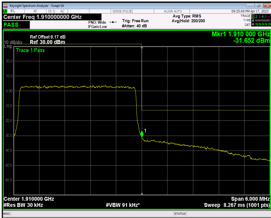
Band2 QPSK BW=5MHz Channel=18625 RB Size=1 Position=#0
