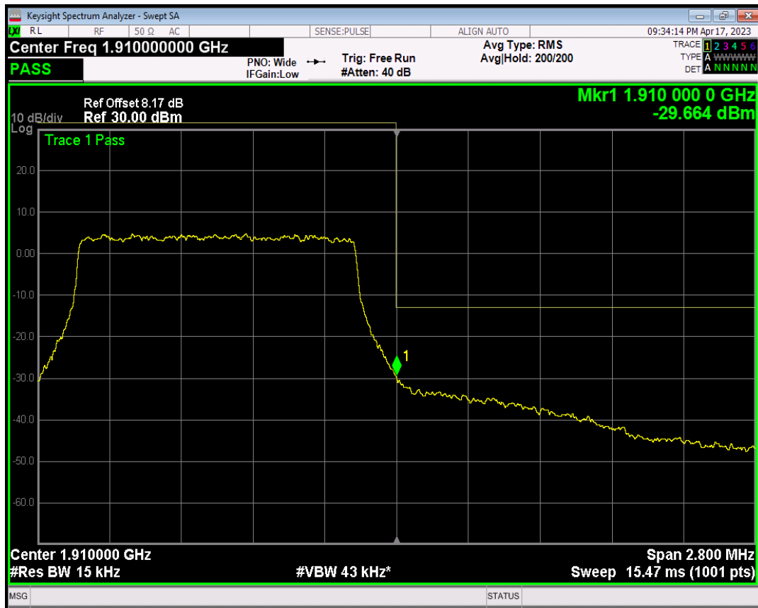
Band2 QPSK BW=3MHz Channel=18615 RB Size=1 Position=#0
