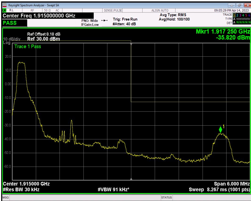
Band25 QAM16 BW=3MHz Channel=26675 RB Size=1 Position=#Max
