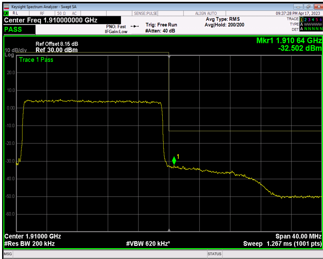
Band2 QAM16 BW=20MHz Channel=19100 RB Size=1 Position=#0
