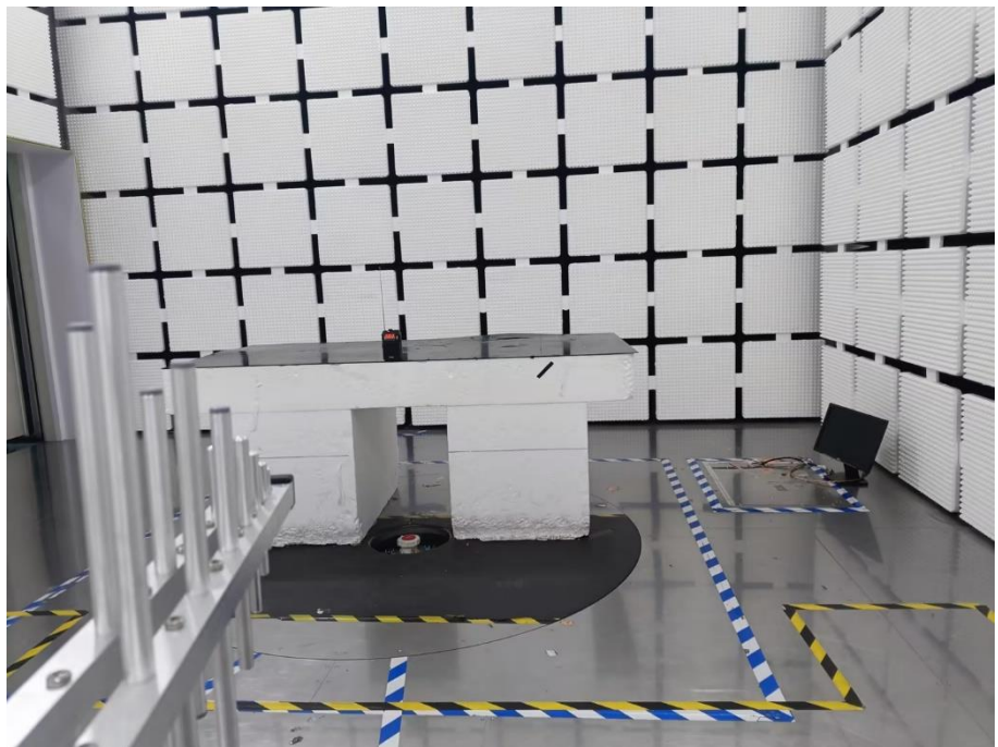
Radiation Emission Test Setup (30MHz to 1GHz)
