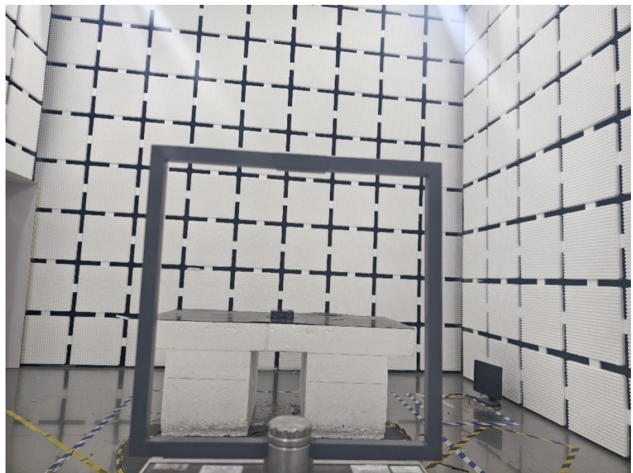
Radiation Emission Test Setup (Below 30MHz)
