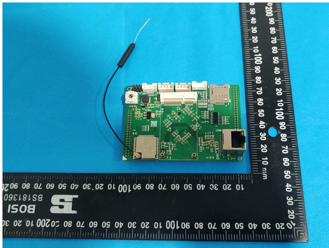
WiFi/BT Module: ESP32-WROOM-32U, FCC ID: 2AC7Z-ESP32WROOM32U, IC:21098-ESP32WROOM32U
