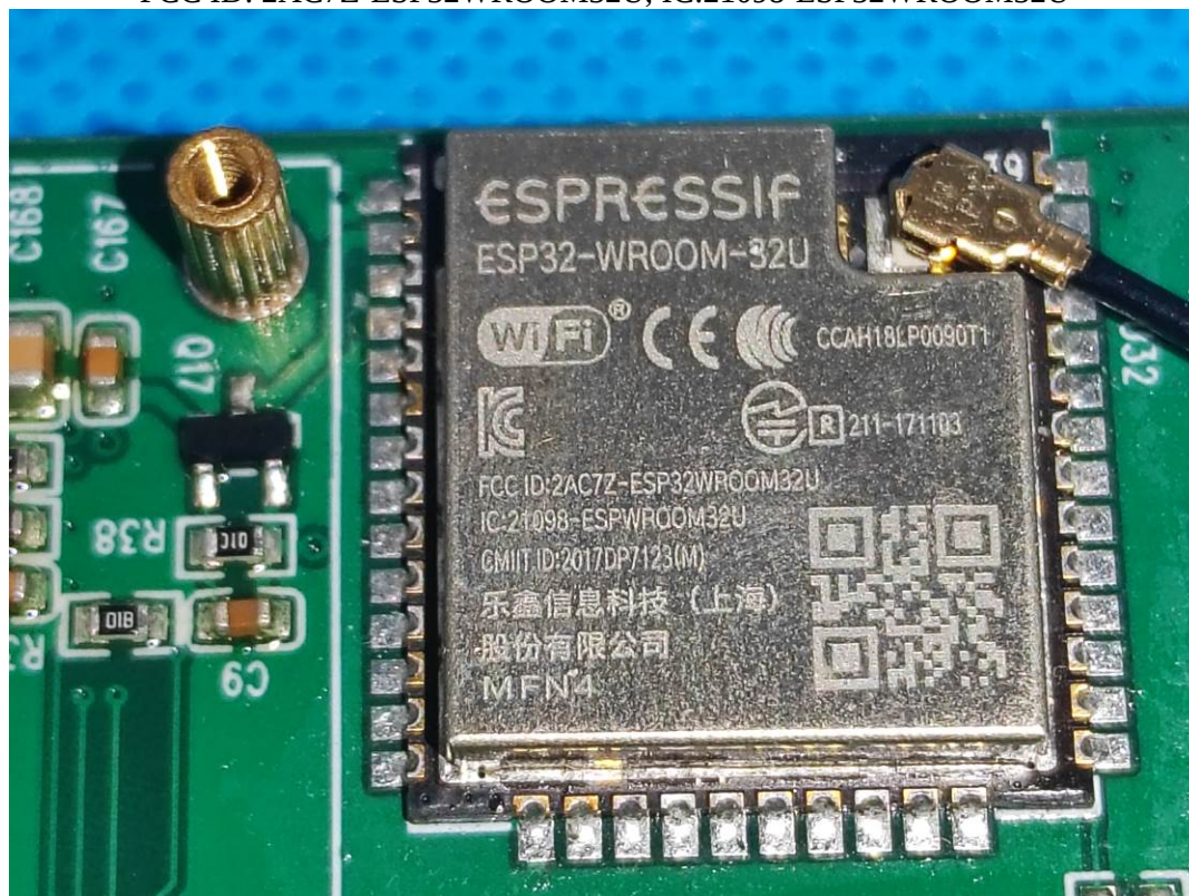
WiFi/BT Module: ESP32-WROOM-32U, FCC ID: 2AC7Z-ESP32WROOM32U, IC:21098-ESP32WROOM32U
