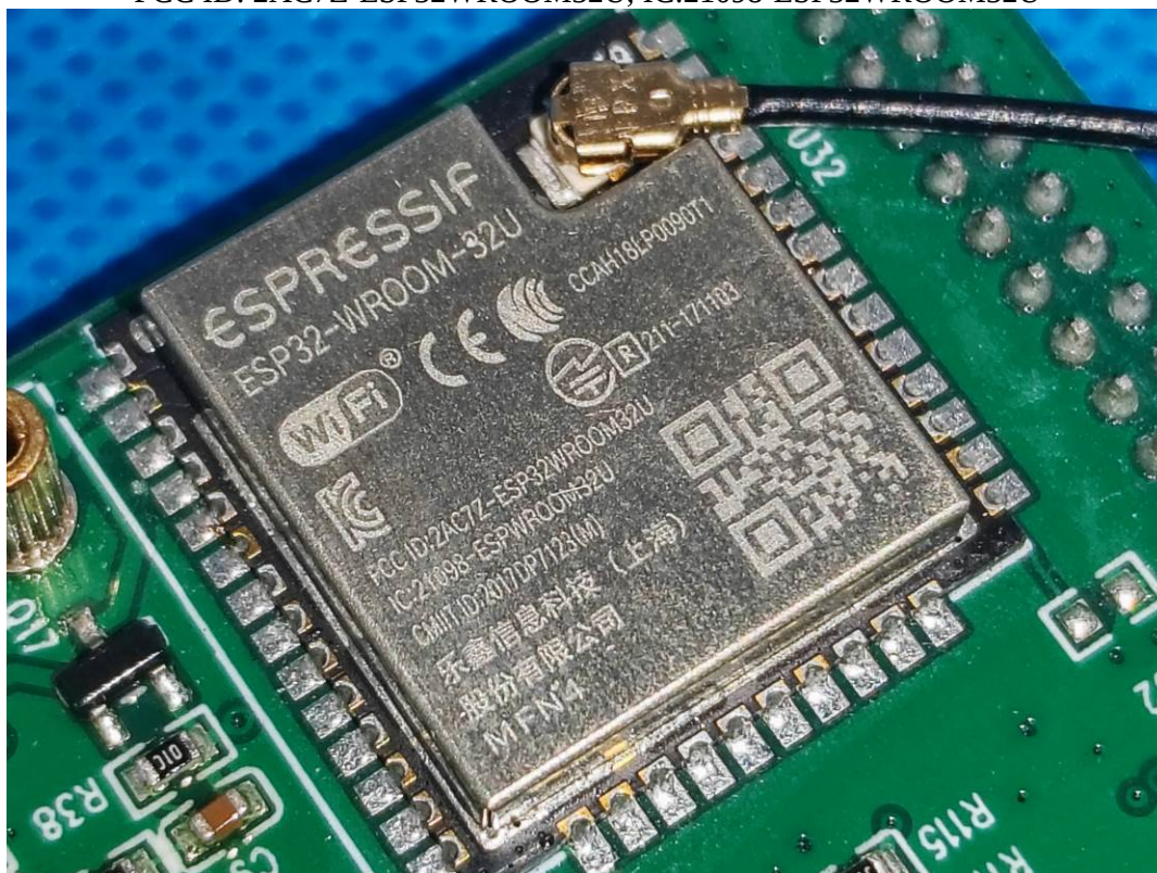
WiFi/BT Module: ESP32-WROOM-32U, FCC ID: 2AC7Z-ESP32WROOM32U, IC:21098-ESP32WROOM32U
