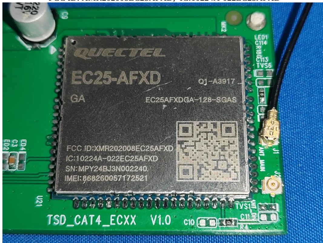
WWAN Module: EC25-AFXD, FCC ID: XMR202008EC25AFXD, IC:10224A-022EC25AFXD
