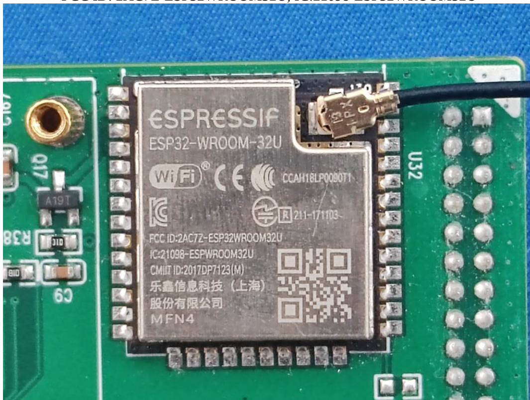
WiFi/BT Module: ESP32-WROOM-32U, FCC ID: 2AC7Z-ESP32WROOM32U, IC:21098-ESP32WROOM32U
