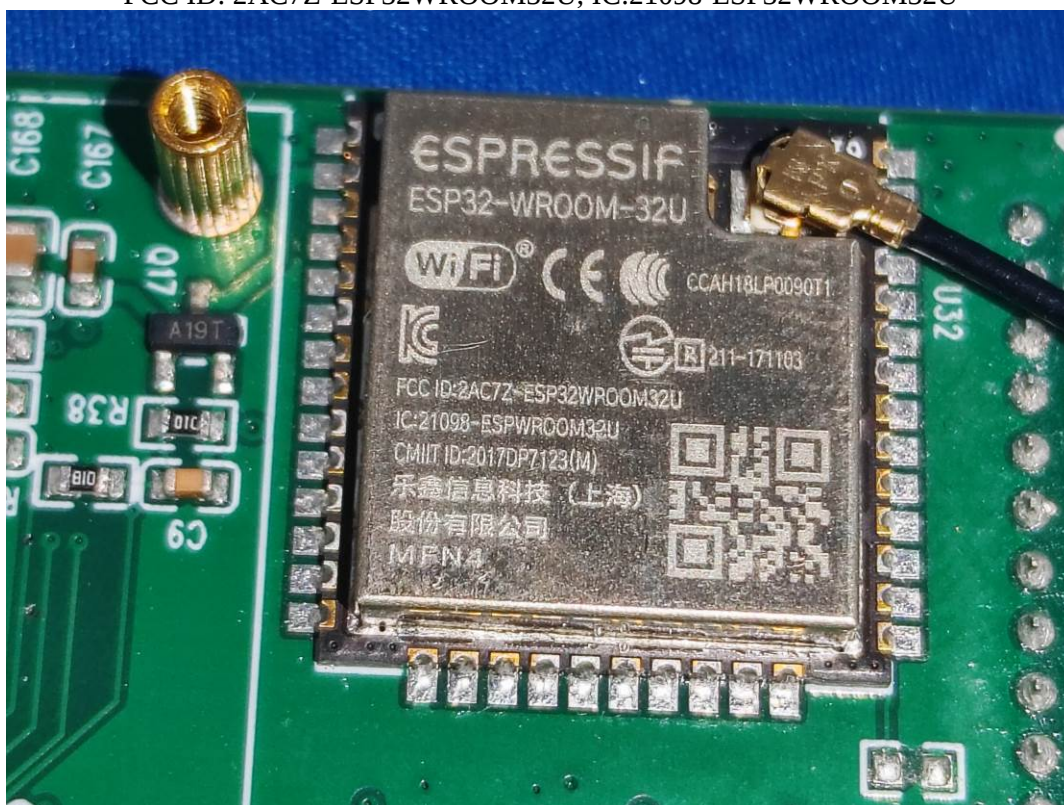
WiFi/BT Module: ESP32-WROOM-32U, FCC ID: 2AC7Z-ESP32WROOM32U, IC:21098-ESP32WROOM32U
