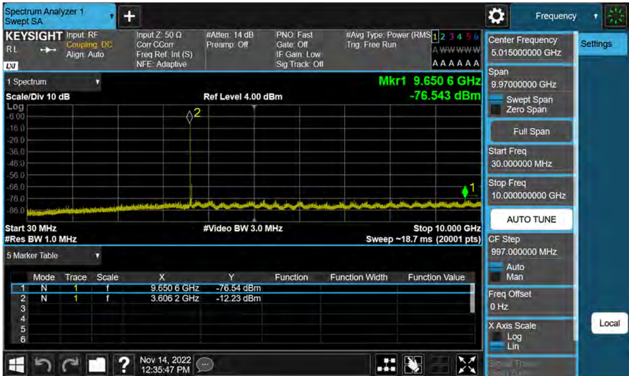
Sub6 n48. Conducted Spurious Plot 1 (40 MHz Ch. 641666 BPSK RB 1, Offset 1)
