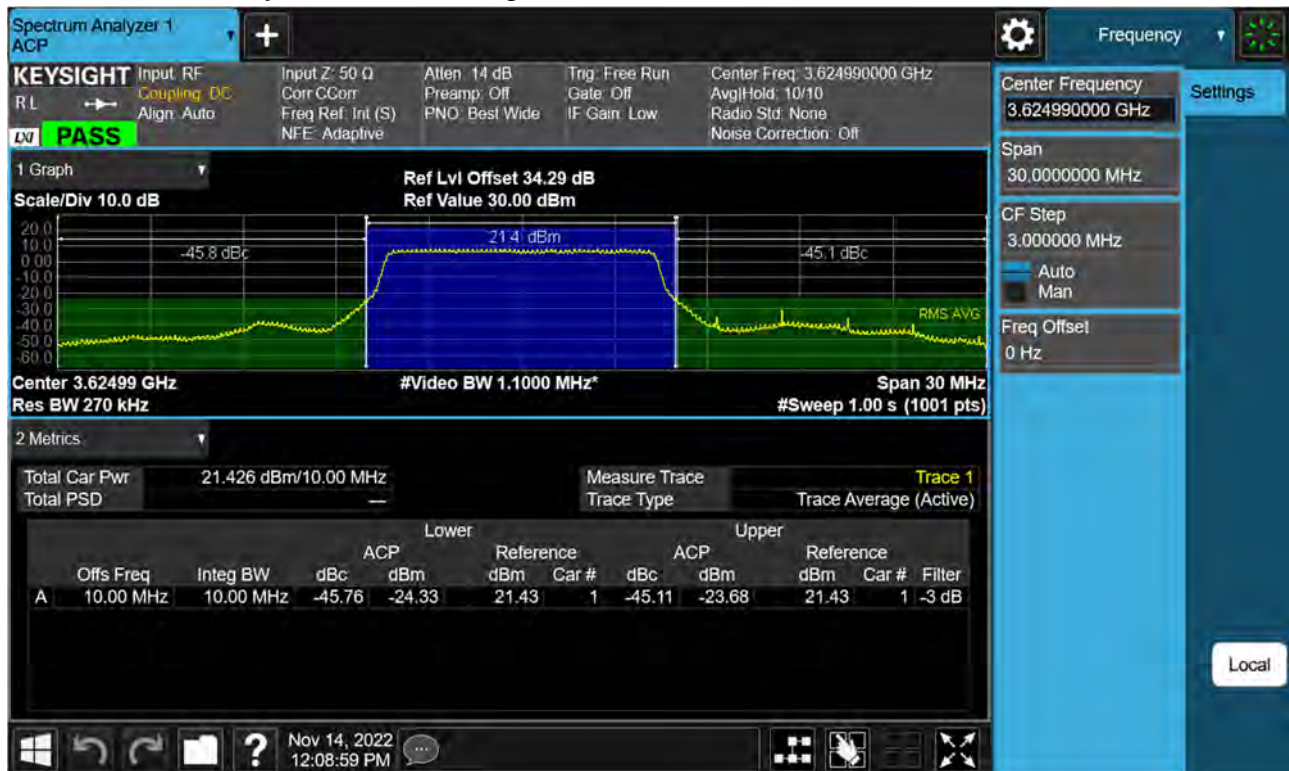
Sub6 n48. Adjacent Channel Leakage Ratio(ACLR) Plot (10 MHz Ch.641666 BPSK RB 24, Offset 0)
