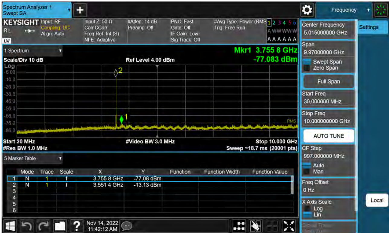
Sub6 n48. Conducted Spurious Plot 1 (30 MHz Ch. 637668 BPSK RB 1, Offset 1)
