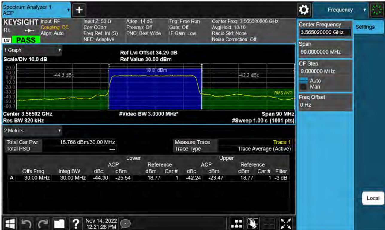
Sub6 n48. Adjacent Channel Leakage Ratio(ACLR) Plot (30 MHz Ch.638000 BPSK RB 75, Offset 0)
