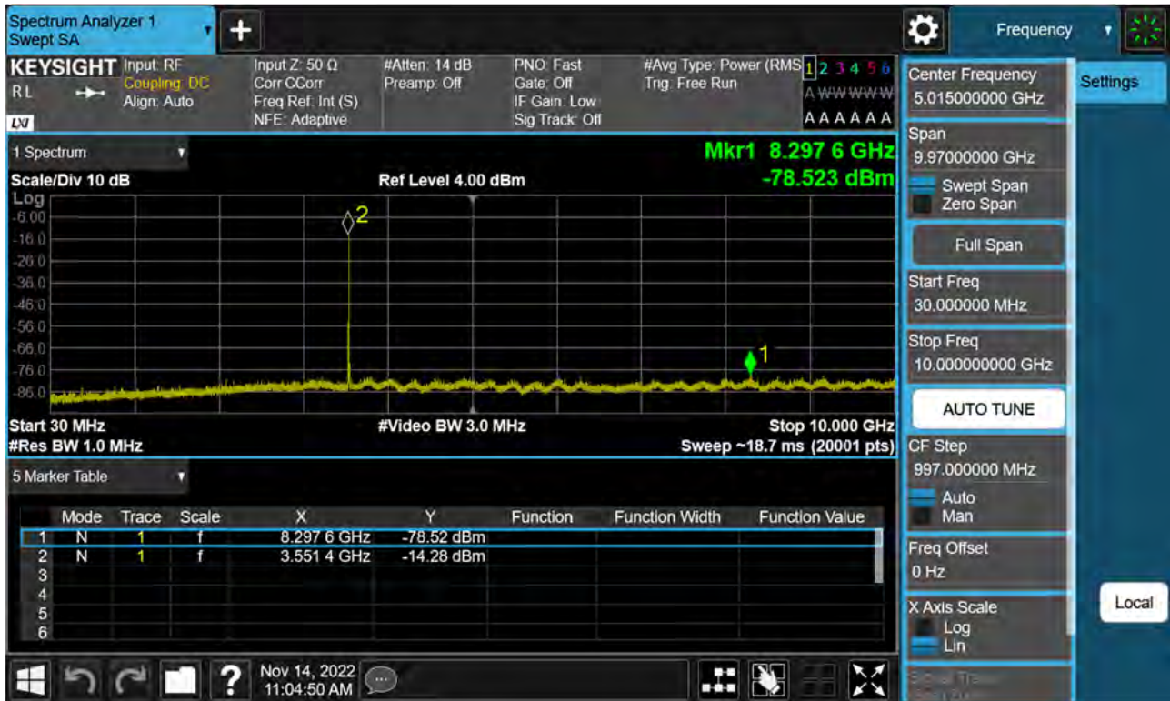
Sub6 n48. Conducted Spurious Plot 1 (10 MHz Ch. 637000 BPSK RB 1, Offset 1)
