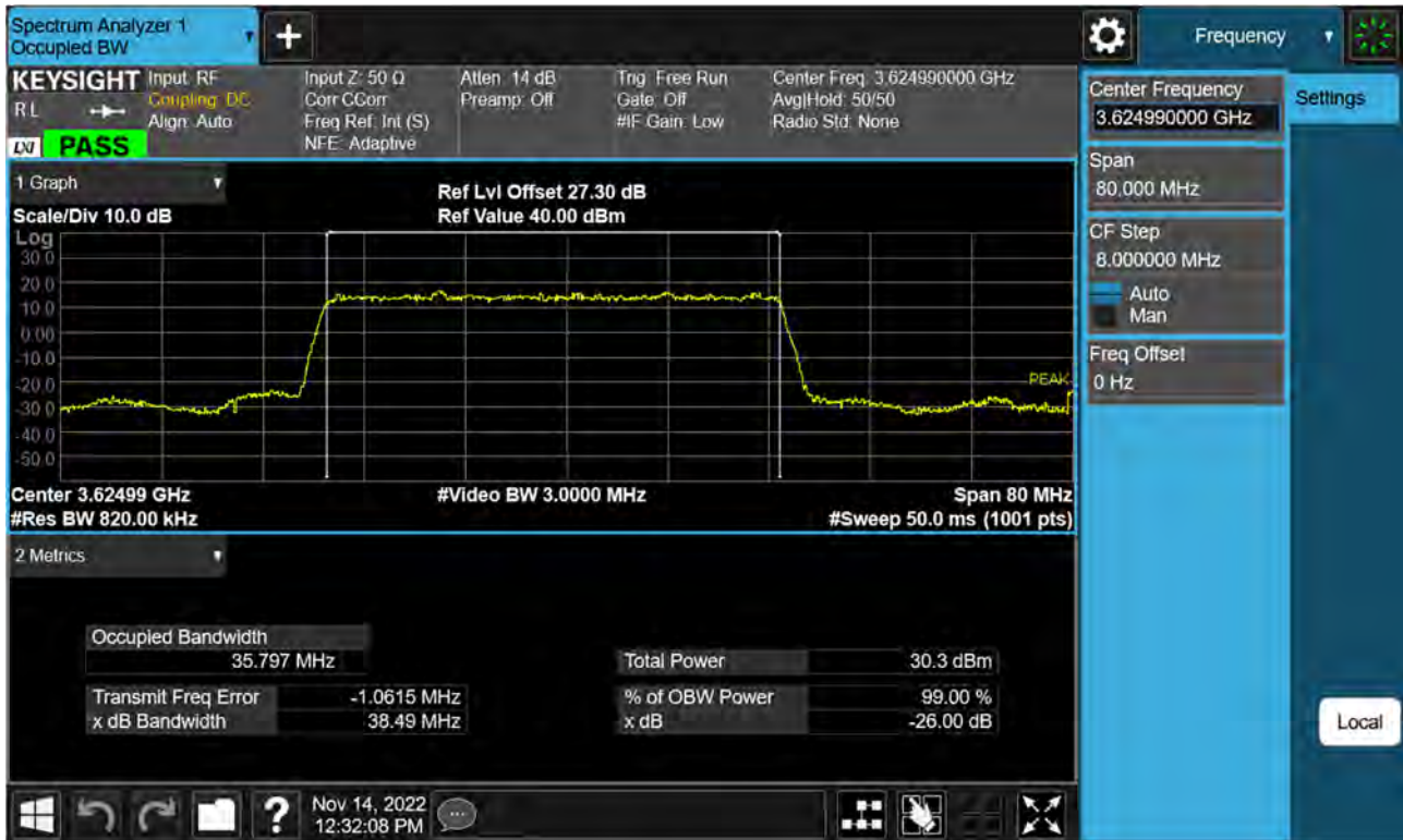
Sub6 n48. Occupied Bandwidth Plot (40 MHz Ch. 641666 BPSK RB 100)
