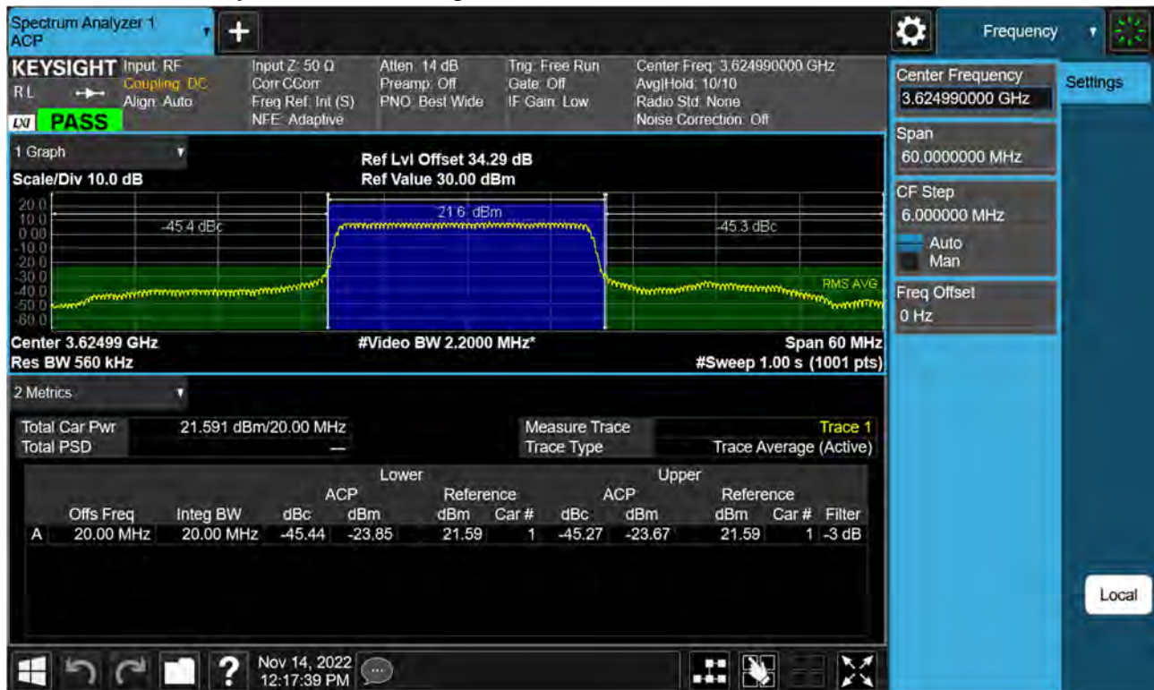
Sub6 n48. Adjacent Channel Leakage Ratio(ACLR) Plot (20 MHz Ch.641666 BPSK RB 50, Offset 0)
