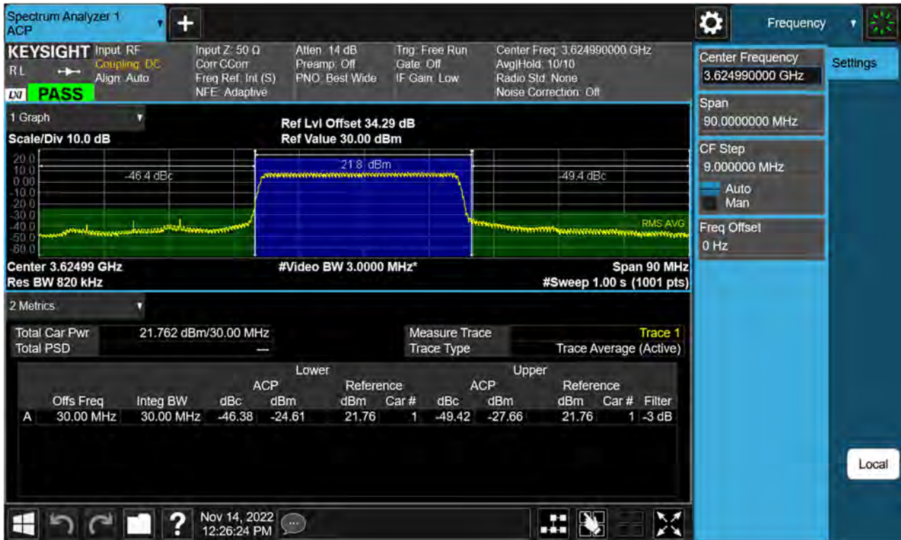
Sub6 n48. Adjacent Channel Leakage Ratio(ACLR) Plot (30 MHz Ch.641666 BPSK RB 75, Offset 0)
