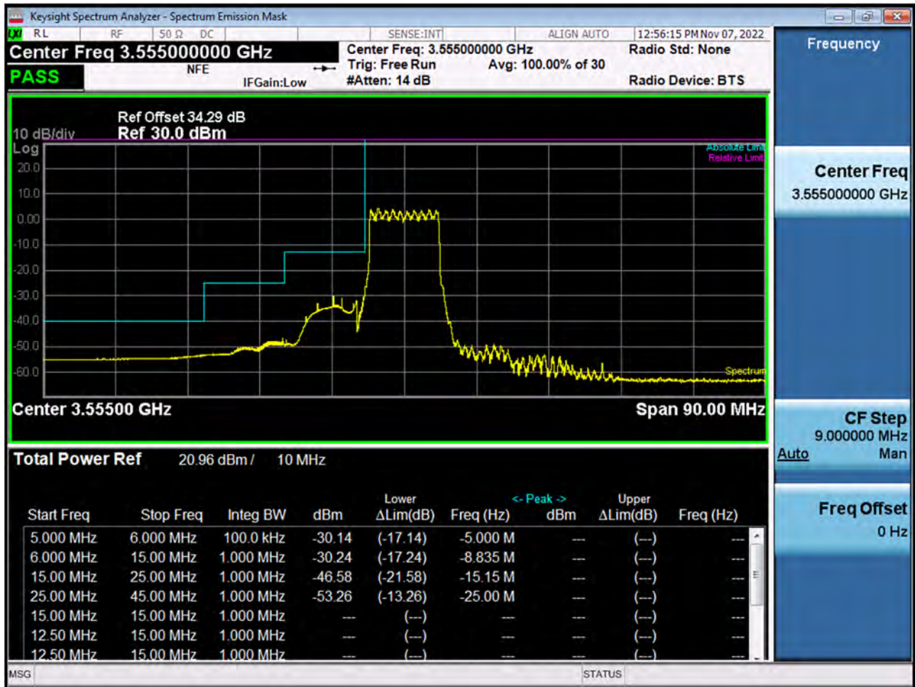
Sub6 n48. 10 M BandEdge(Lower)_Low_3555.00 MHz_BPSK_FullIRB
