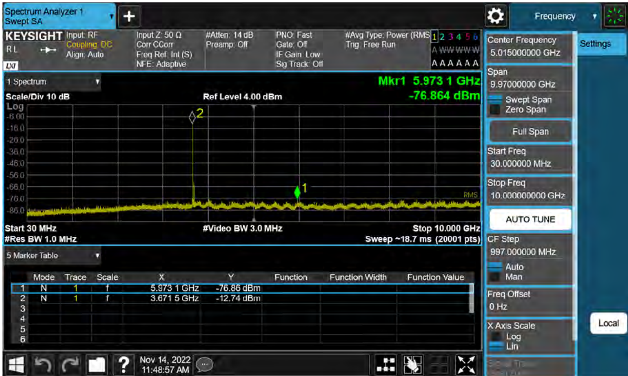
Sub6 n48. Conducted Spurious Plot 1 (30 MHz Ch. 645666 BPSK RB 1, Offset 1)
