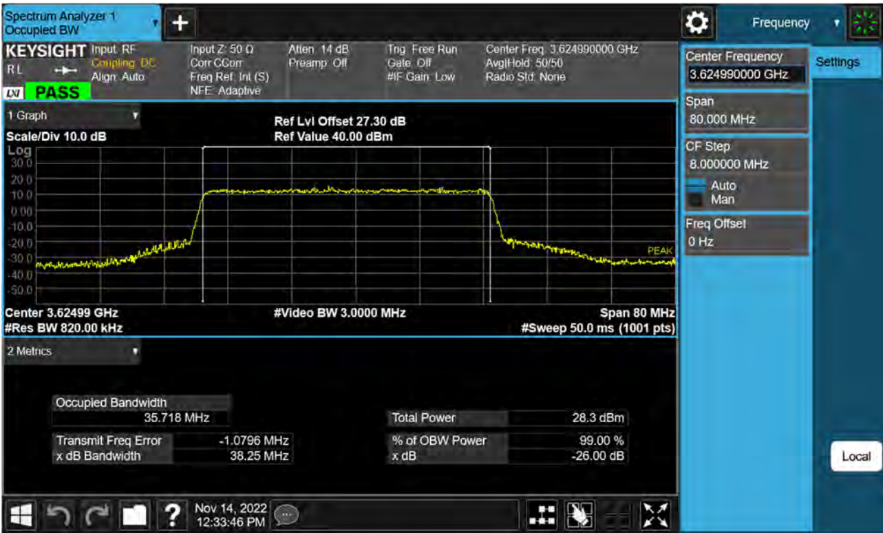
Sub6 n48. Occupied Bandwidth Plot (40 MHz Ch.641666 64-QAM RB 100)
