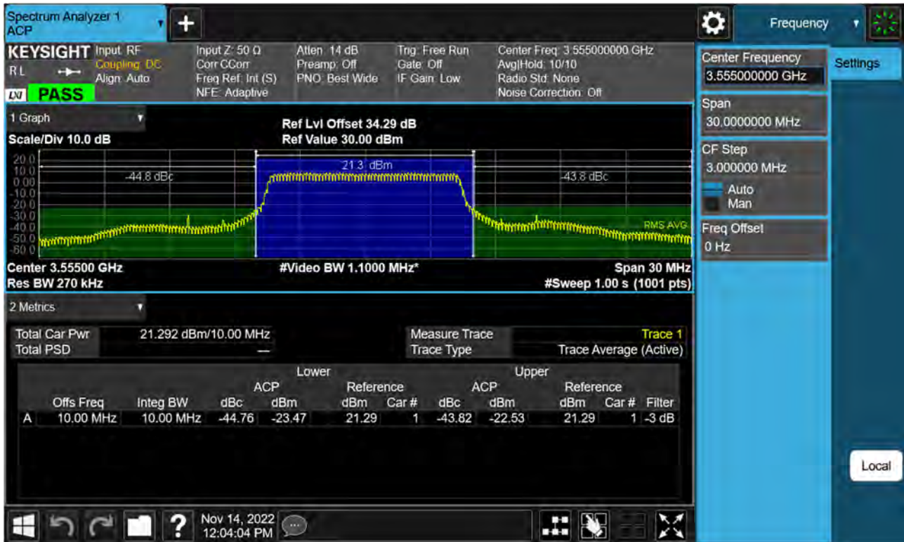
Sub6 n48. Adjacent Channel Leakage Ratio(ACLR) Plot (10 MHz Ch.637000 BPSK RB 24, Offset 0)
