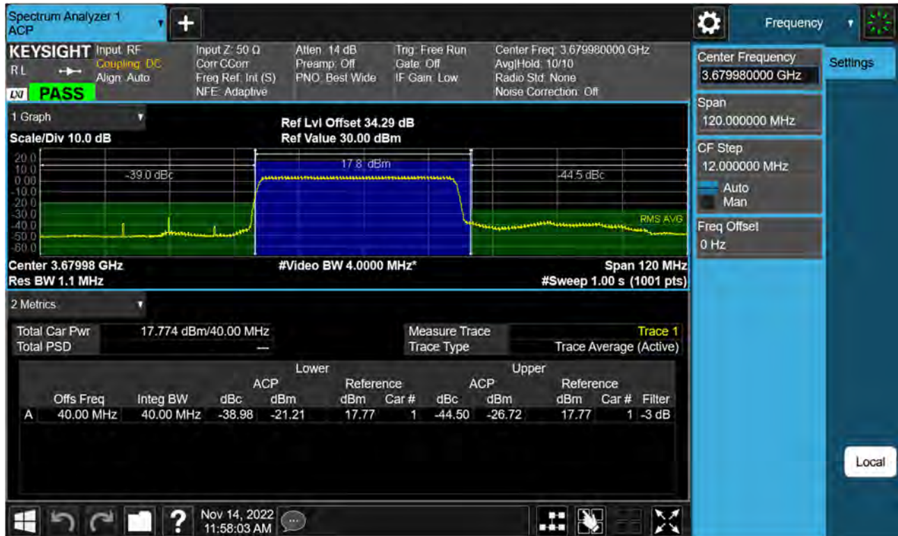
Sub6 n48. Adjacent Channel Leakage Ratio(ACLR) Plot (40 MHz Ch.645332 BPSK RB 100, Offset 0)
