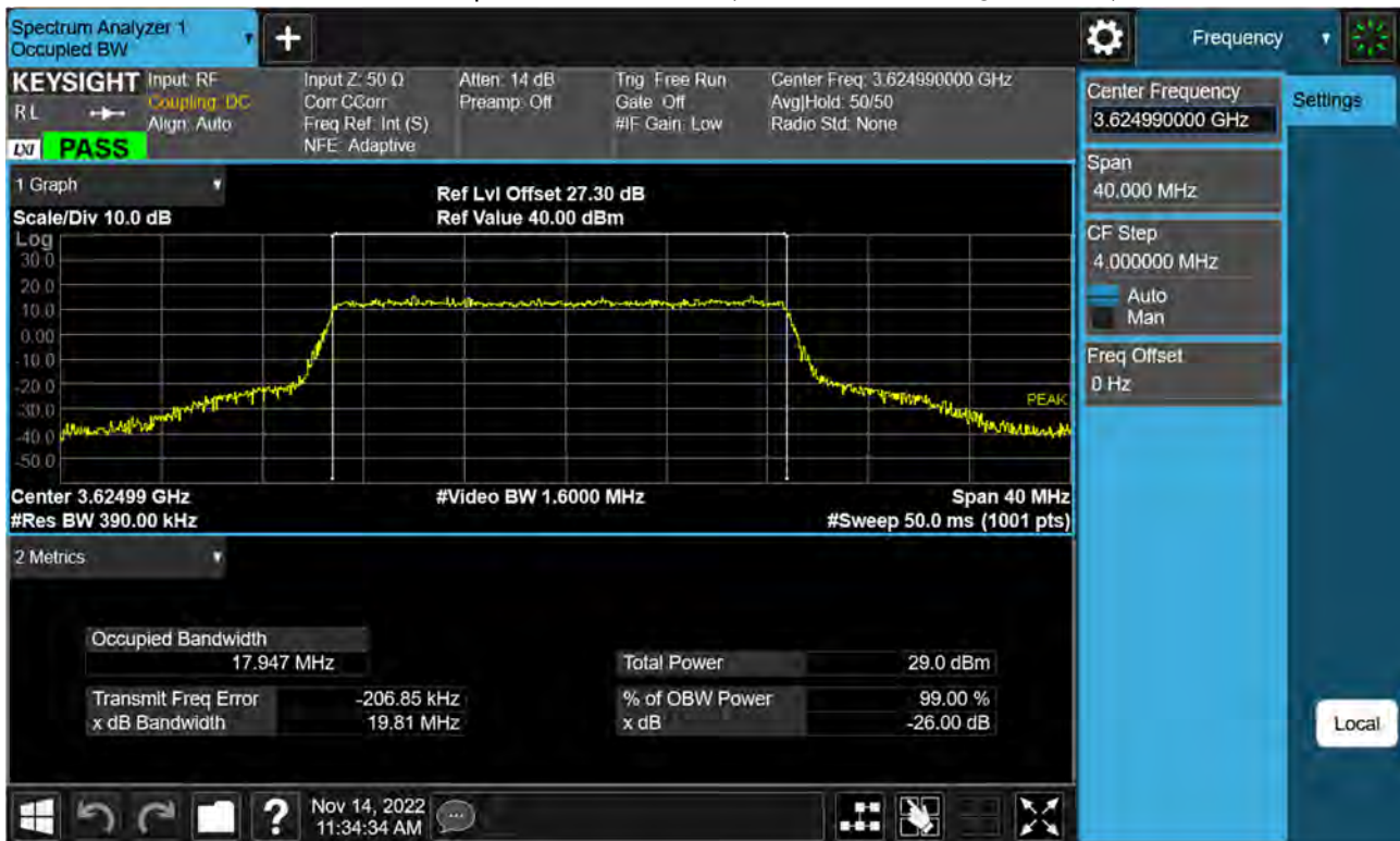
Sub6 n48. Occupied Bandwidth Plot (20 MHz Ch. 641666 QPSK RB 50)
