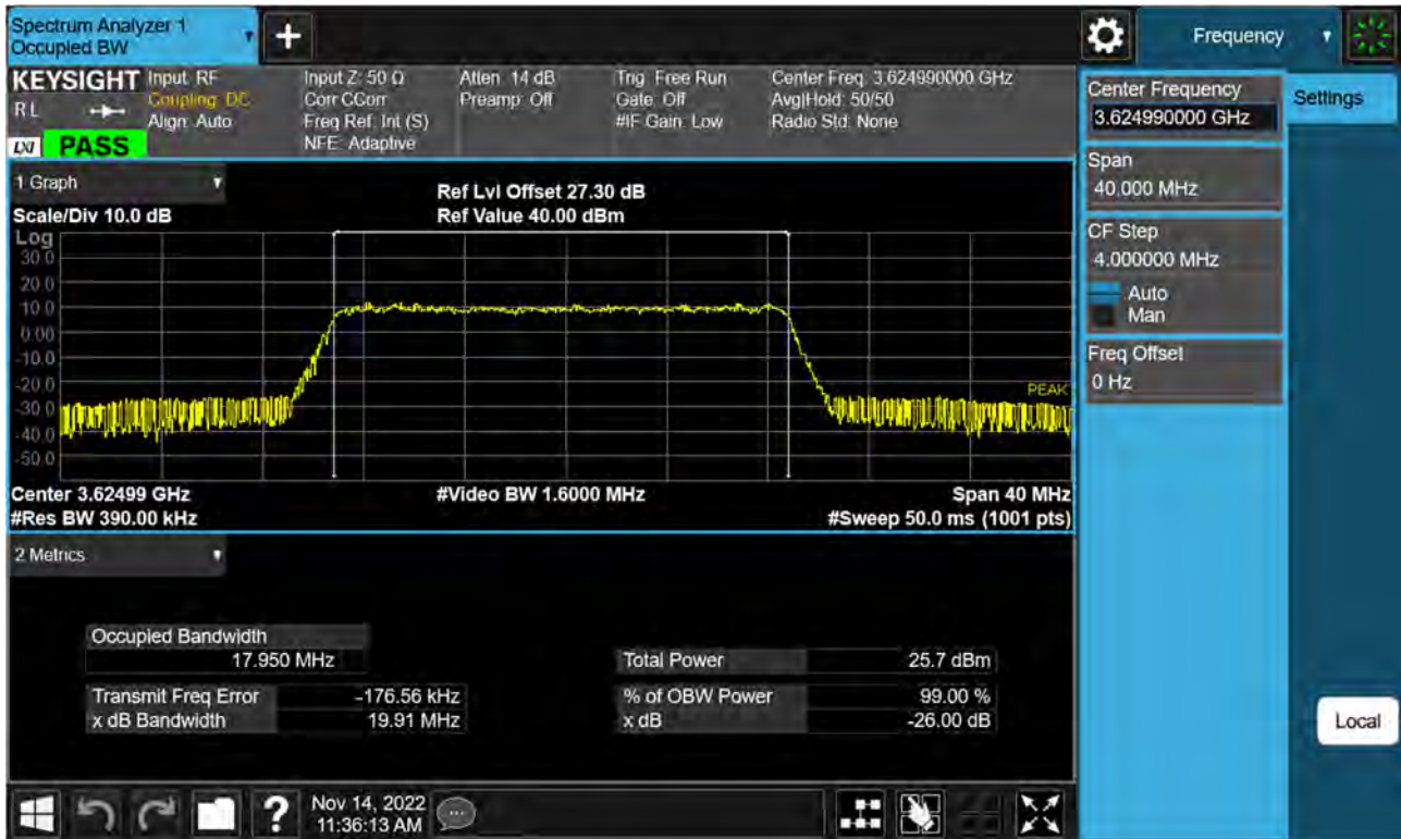
Sub6 n48. Occupied Bandwidth Plot (20 MHz Ch.641666 256-QAM RB 50)
