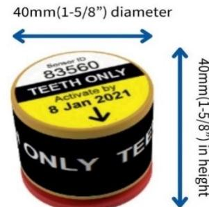
The SEN\_GET\_P1\_5.5 is a consumable RFID sensor tag for the GET Trakka breakage detection solution. Designed to be embedded inside Ground Engaging Tools for active monitoring of digger wear components during operation and built for extreme mining conditions. This SEN\_GET\_P1\_5.5 wirelessly transmits data to the receiver via RF transmissions and is activated/deactivated using the portable reader.
