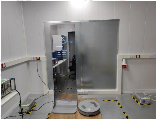
Radiated Emissions for 30MHz~1GHz
