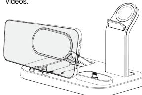
3 To remove the watch charger, press the button on the back to the right and you can easily take it off.
