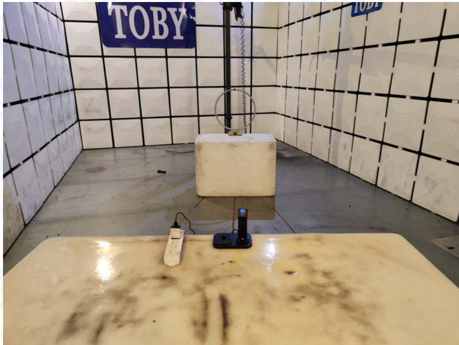
Photo of Setup for Radiated Emission (30MHz~1GHz)
