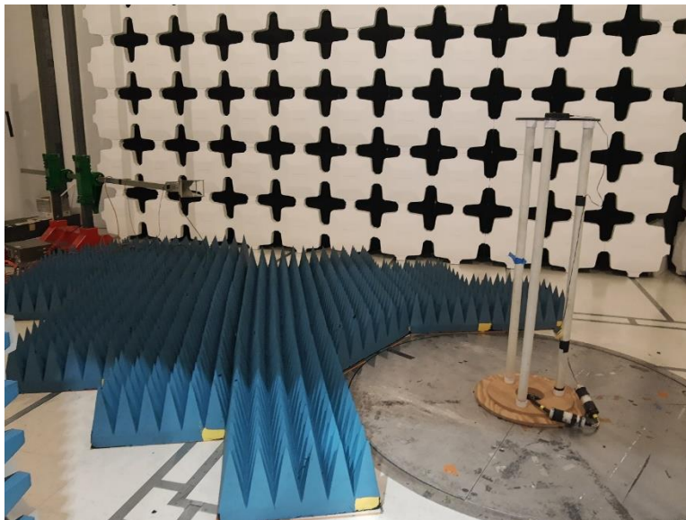
Photograph 4. Radiated Emissions - 1-18GHz Test Setup
