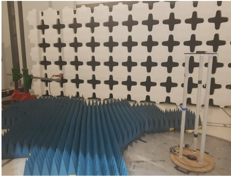
Photograph 5. Radiated Emissions - 18-25GHz Test Setup
