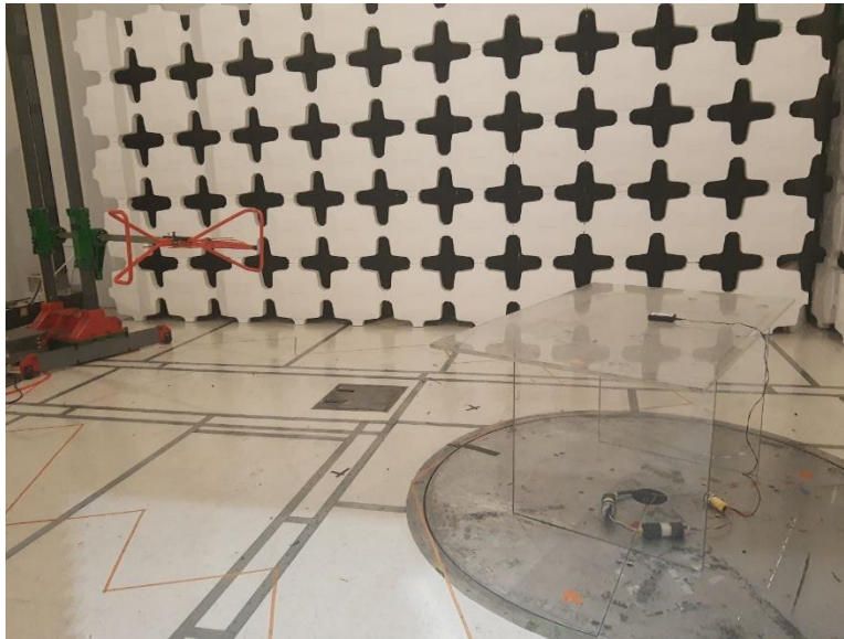
Photograph 3. Radiated Emissions - 30-1000MHz Test Setup
