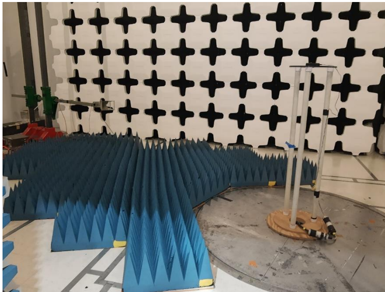
Photograph 4. Radiated Emissions - 1-18GHz Test Setup
