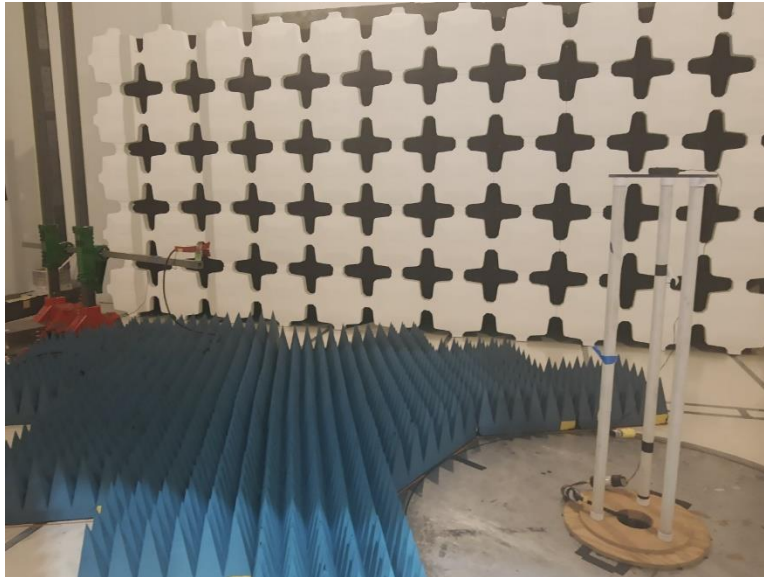
Photograph 5. Radiated Emissions - 18-25GHz Test Setup
