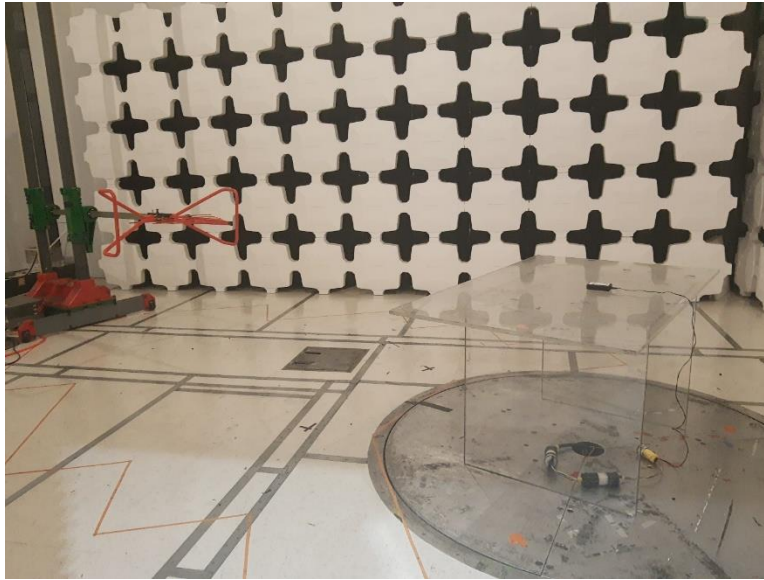
Photograph 3. Radiated Emissions - 30-1000MHz Test Setup
